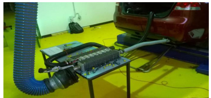
Figure 13. Prototype of combined HP-TEG heat recovery system [39].
