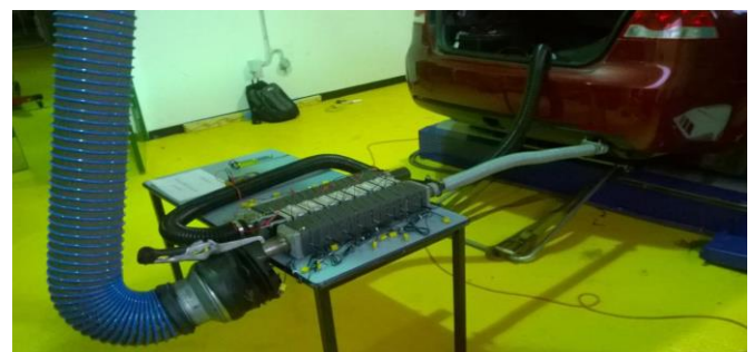
Figure 13. Prototype of combined HP-TEG heat recovery system [39].
