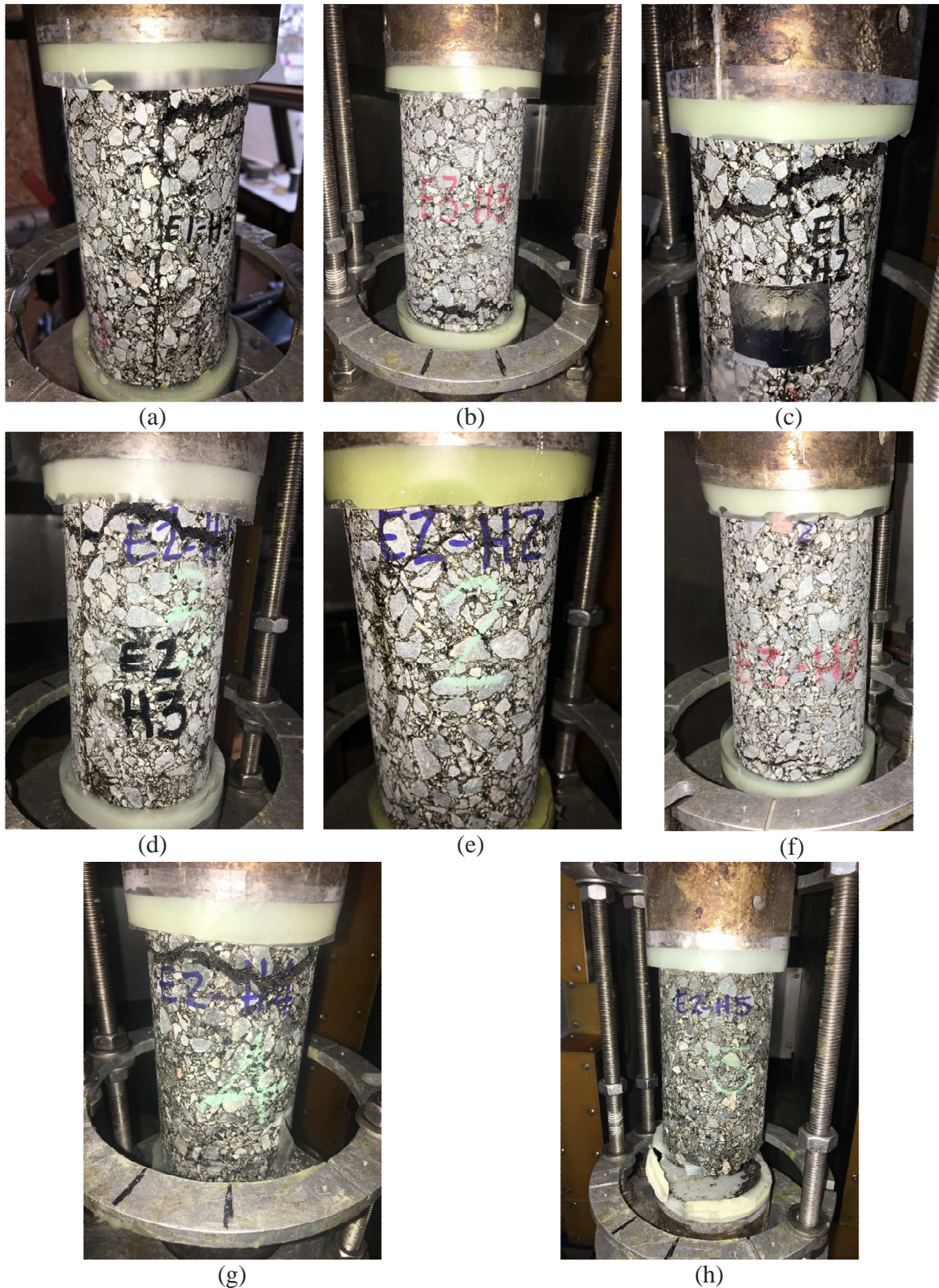
Figure B2-6. Tested specimens of configuration E, type H: (a) E1-H3, 40°C and 2%/min, (b) E3-H3, 40°C and 2%/min, (c) E1-H2, 19°C and 2%/min, (d) E2-H3, 19°C and 2%/min, (e) E2-H2, 19°C and 0.004%/min, (f) E3-H2, 19°C and 0.003%/min, (g) E2-H4, 0°C and 0.003%/min, (h) E2-H5, 0°C and 0.001%/min
