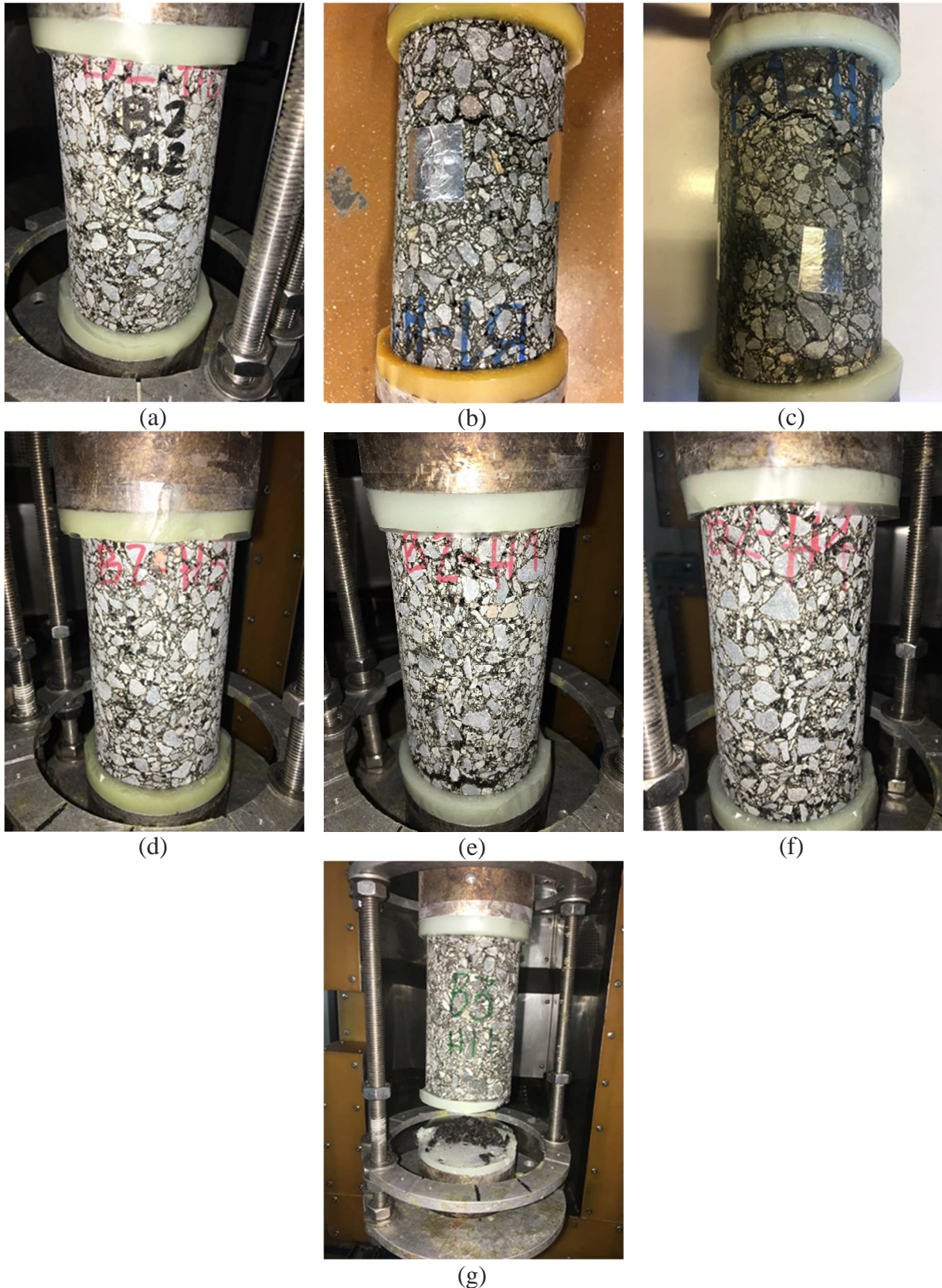
Figure B2-3. Tested specimens of configuration B, type H: (a) B1-H1, 40°C and 2%/min, (b) B2-H2, 40°C and 2%/min, (c) B1-H2, 19°C and 2%/min, (d) B2-H3, 19°C and 2%, (e) B2-H1, 19°C and 0.005%/min, (f) B2-H4, 19°C and 0.004%/min, (g) B3-H11, 0°C and 0.001%/min
