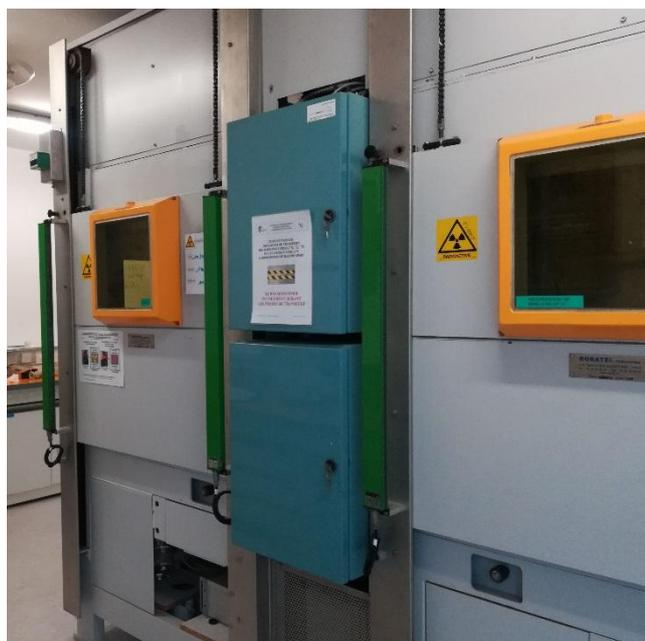
Figure 110 : Photos of: (left) fumehood with lead-shielded wall (right) hot cell
