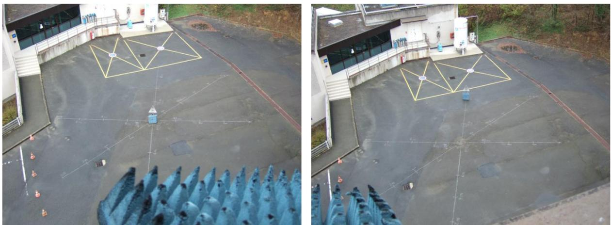
**Figure 63: static targets (left) calibrator position (right) calibrator placed at 5.197meter from the calibrator on the  $0^\circ$  axis**
