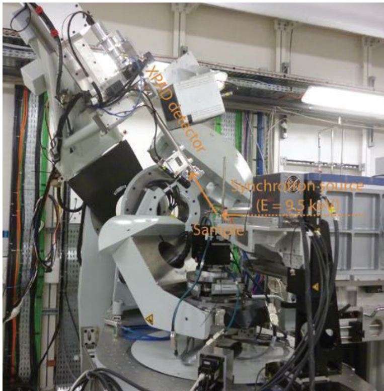
Figure A.20: Experimental setup of ADXRD at DIFFABS beamline.
