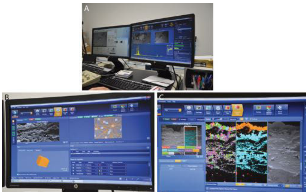
Figure 3.28: Photos of data processing. A, Treatment of EDS data using the Quantax 400 software. B and C, Treatment of EBSD data using the Aztec HKL software.
