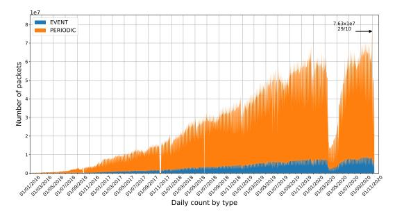
Figure 5.10: Evolution of transmitted CVs packets throughout the years.
