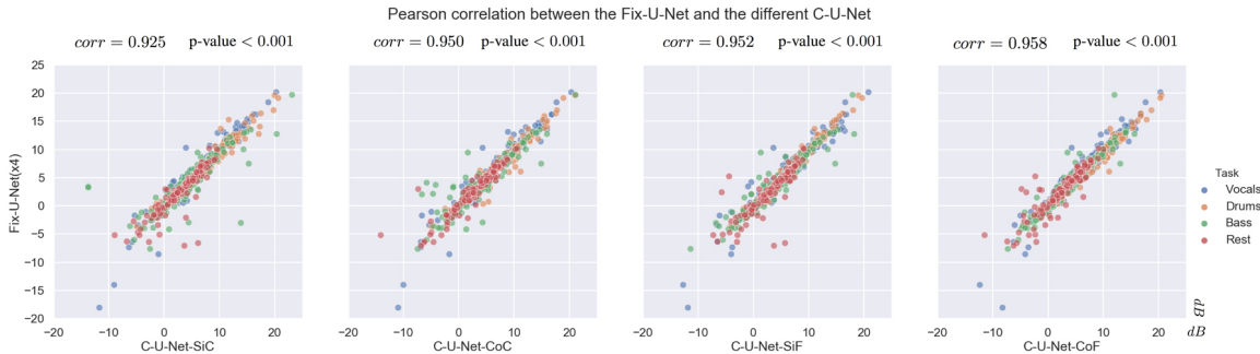
Figure 8.5: Each graph correlates the performance of two models. On top of it, we show the correlation and p-value. The 'y' axis represents the fixed version (the four separated U-Nets) and the 'x' one a different C-U-Net version (with progressive train). The coordinates of each dots correspond to the models' performance i.e., 'y' position for the Fix-U-Net performance and 'x' for C-U-Net. There are three dots per song, one per metric (SIR, SAR, and SDR) which does a total of 600 (50 songs x 3 metrics x 4 instruments). The dot alignment in the diagonal implies a strong correlation between models: if one works well, so do the others, and vice versa. Each color highlights the points of each source separation task.
