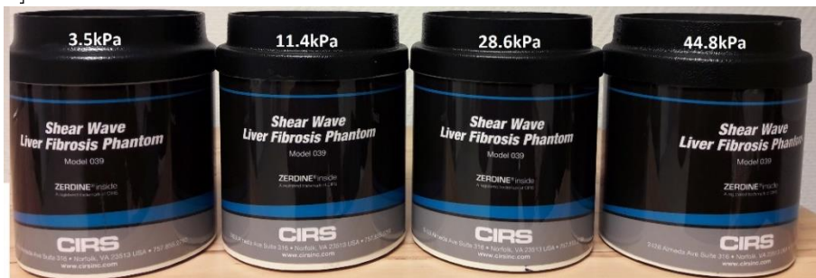
Figure 2.2.1: Set of CIRS test phantoms {C1,C2,C3,C4} calibrated for liver fibrosis staging and grading at 3.5 kPa, 11.4 kPa, 28.6 kPa, and 44.8 kPa.
