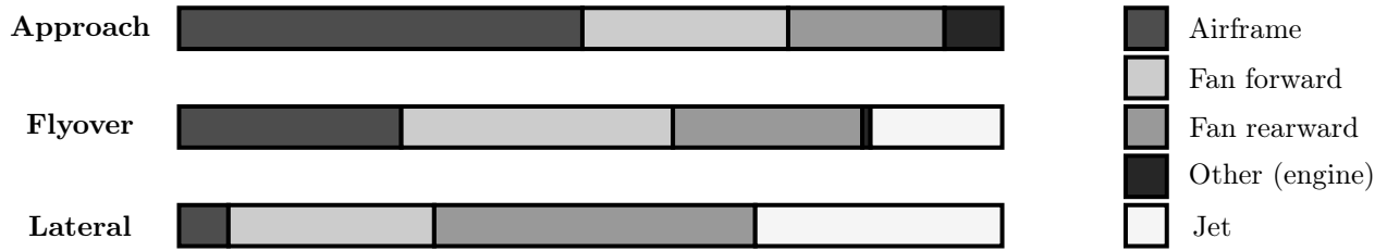
Figure 1.3: Noise sources breakdown at certification points for a modern middle-range commercial aircraft (Lempereur, 2018).
