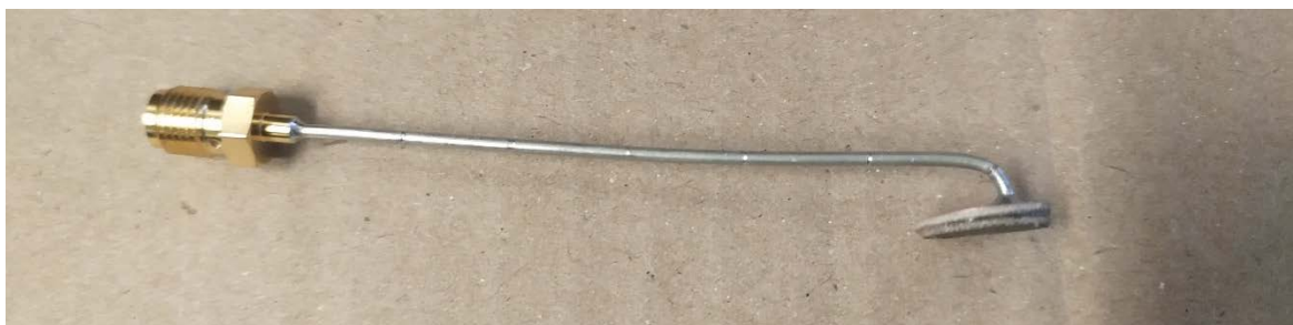
Figure 5.14 Soldered and bent antenna
