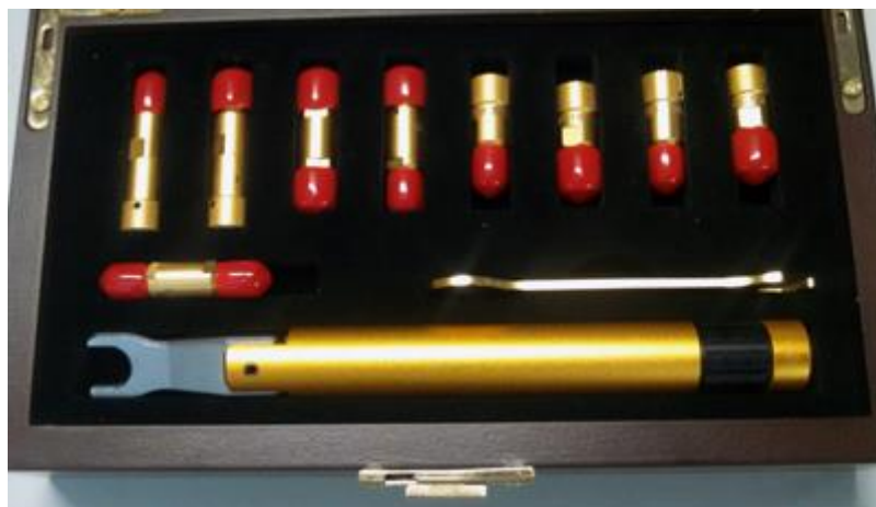
Figure 5.2 Calibration kit of the VNA
