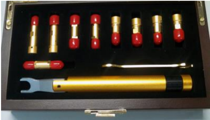
Figure 5.2 Calibration kit of the VNA
