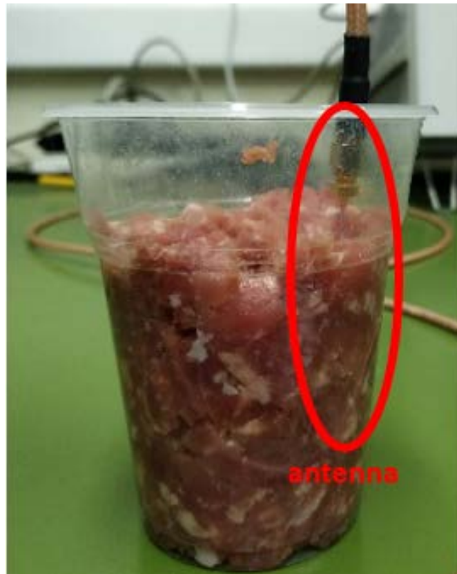
Figure 5.10 Antenna embedded together with the coaxial connector
