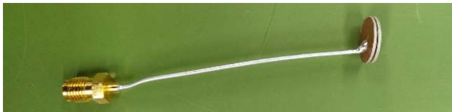
Figure 5.9 Antenna soldered with the coaxial connector
