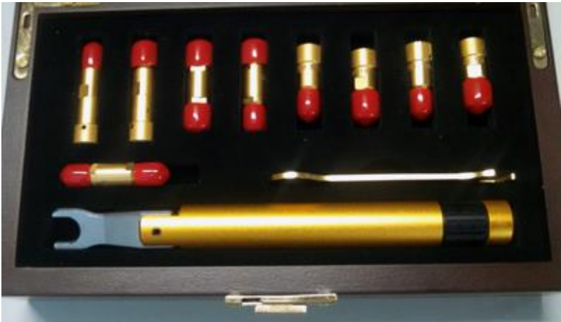
Figure 5.2 Calibration kit of the VNA
