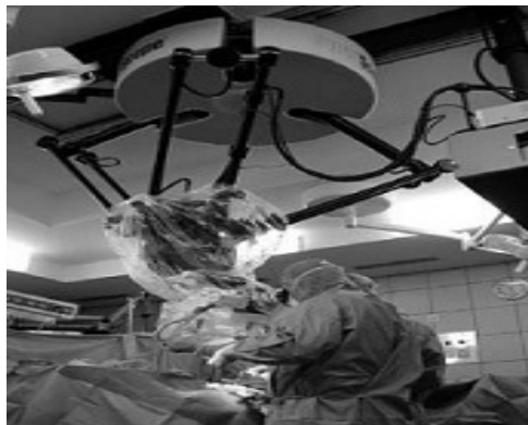
Figure 1.3: ISIS/SurgiScope system using a Delta robot as microscope stand
