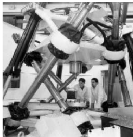
Figure 1.8: The Variax of Giddings and Lewis, the first industrial parallel milling machine presented in 1994 at IMTS [Merlet 2006]
