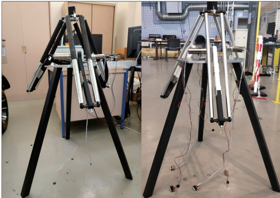
Figure 4.4: Real prototype in front view; left: Prototype 1 for line-based visual servoing, right: prototype 2 for image moment visual servoing
