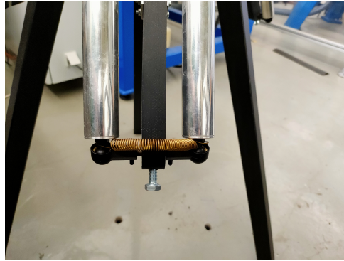
Figure 4.6: Spring fixed on the parallelogram structure of the prototype
