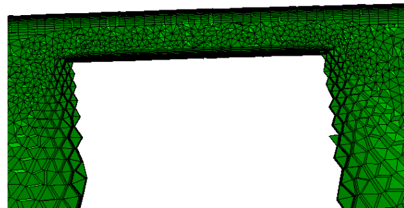
Figure 2.7: Rotor-blade tip-gap mesh, RANS simulation.
