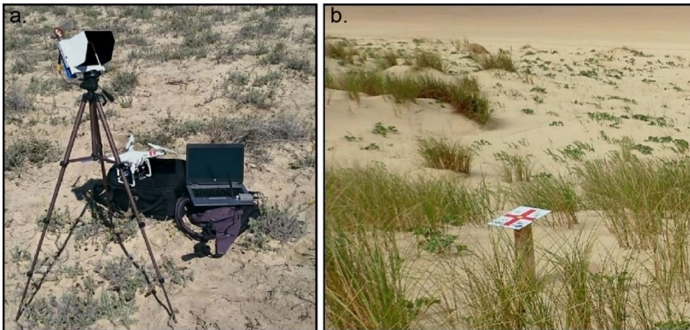
Figure 4.3. The dune survey system composed of (a) light and low-cost UAV hardware, computer ground station, video receiver, and (b) permanent GCPs spaced every 250 m and approximately 50–100 m in the alongshore and cross-shore directions, respectively.
