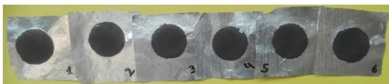
b) Electrodes of LCO:C:PVDF, casted onto 6.5- \mu\text{m} -thick aluminum foils. The latter is used as current collector and to protect the beryllium window.
