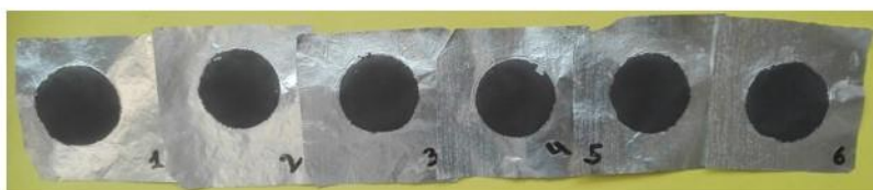
b) Electrodes of LCO:C:PVDF, casted onto 6.5- \mu\text{m} -thick aluminum foils. The latter is used as current collector and to protect the beryllium window.
