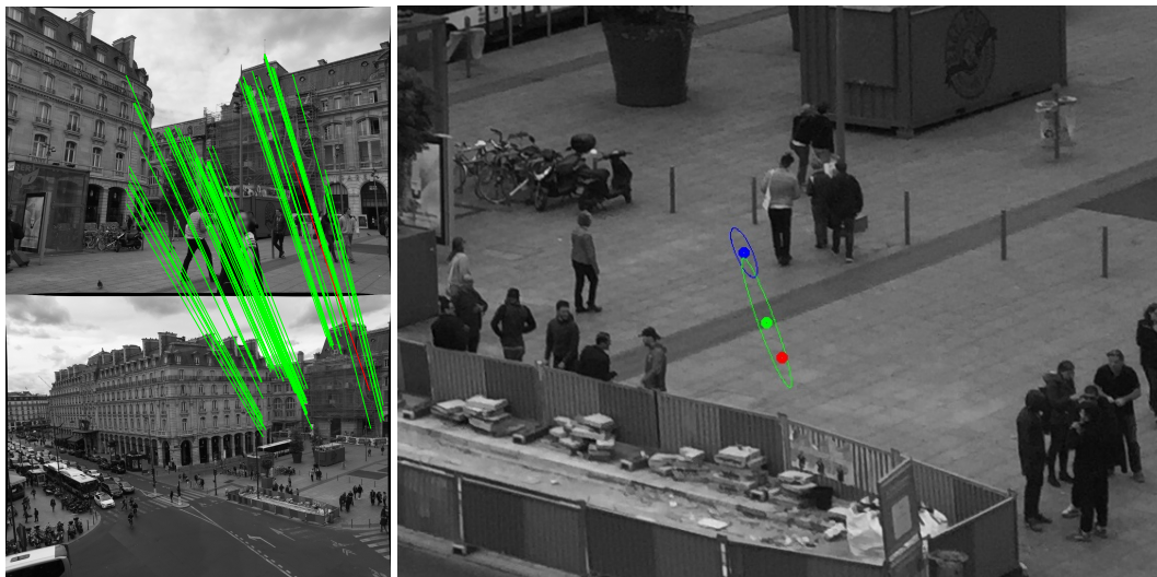
Figure 4.2: Illustration of an epipole uncertainty estimation. For a given pair of images, the matches selected as inliers by RANSAC (91 out of 208 initial matches) are shown with green and red lines. There is only one false positive match which is illustrated by the red line, all the other matches being true positives. In the figure on the right (close-up of the scene in the reference view), the estimated epipole uncertainty on all inliers (presented by blue ellipse) predicts a small standard deviation of the estimated epipole, and misses the true epipole (the red dot). When the single false positive is removed, the epipole ellipse (the green ellipse) predicts the uncertainty in a more reliable way.
