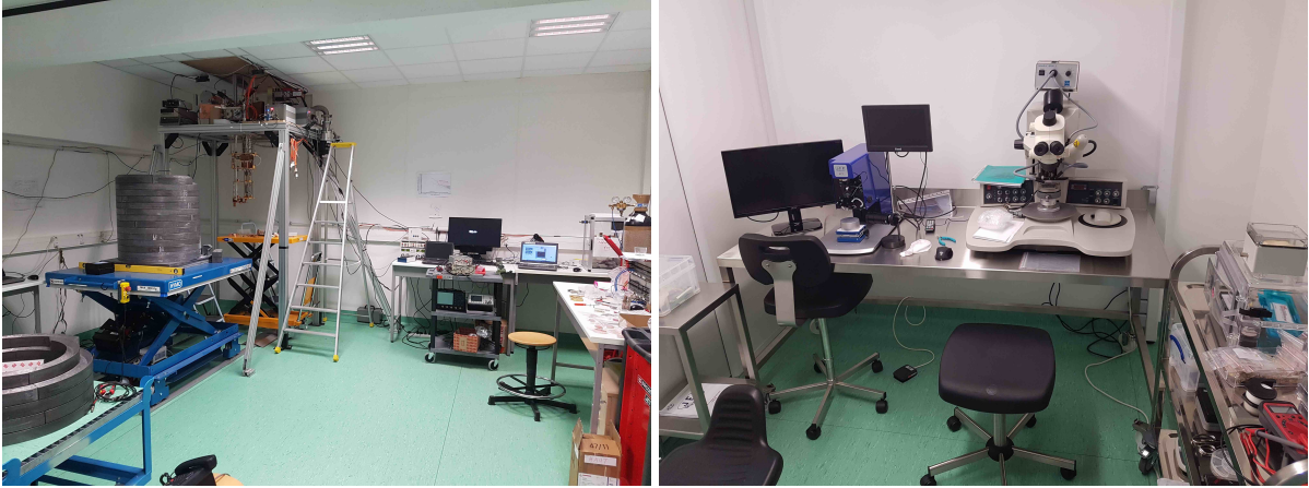
Figure 5.1: Left: Photo of the cryogenic lab, where the dry dilution cryostat (opened) and its lead shield are clearly visible. On the left side are the computers controlling the cryostat, and on the right side are the detector readout and DAQ. Right: Photo of the ISO-5 clean room hosting a wire bonder (right side) and a die bonder (left).
