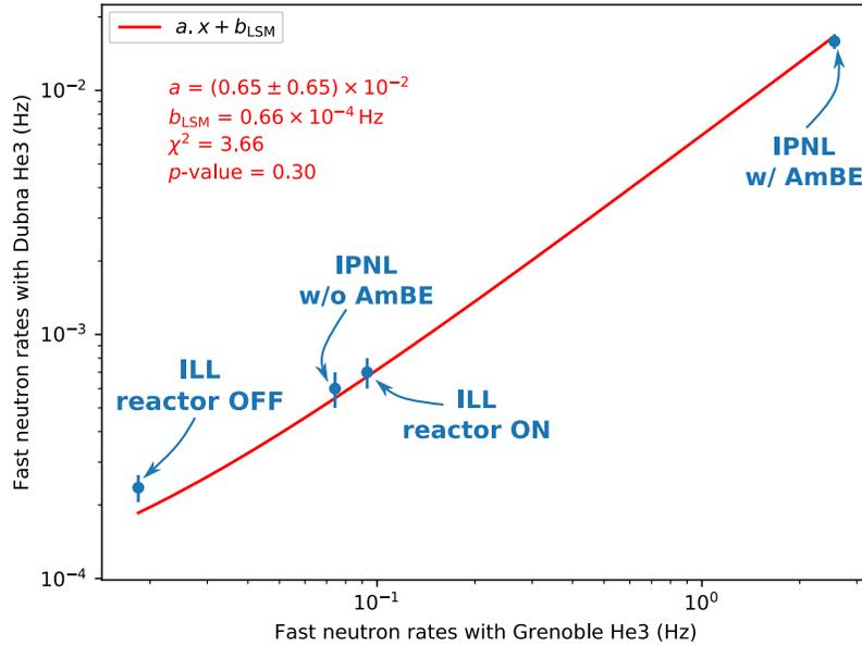
Figure 3.12: Correlation between the fast neutron measurements from the ILL (x-axis) and JINR (y-axis) <sup>3</sup>He PC, realised at the ILL-H7 site and at IP2I.
