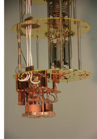
Figure 5.5: New suspended detector tower being commissioned.
