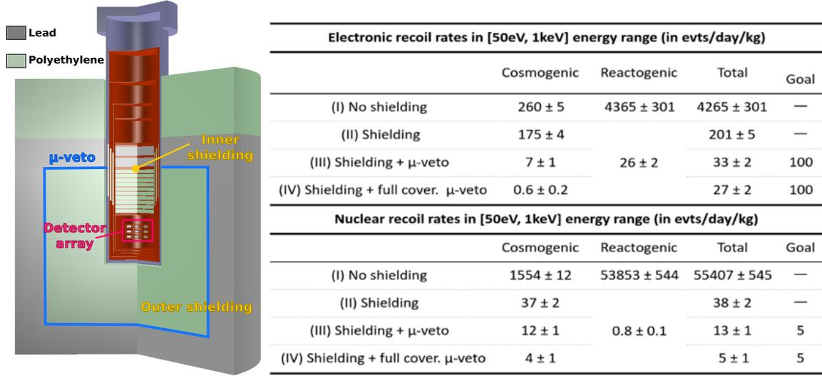
Figure 3.7: **Left:** Preliminary shielding design of the RICOCHET experiment at ILL-H7 considered in the Geant4 simulations. **Right:** Simulated background rates inside the cryogenic detector array for various shielding design scenarios, when only one bolometer has triggered. Scenario (III) corresponds to our preliminary shielding design illustrated on the left panel. The muon-veto (blue) has been modelled assuming a perfect muon tagging efficiency.
