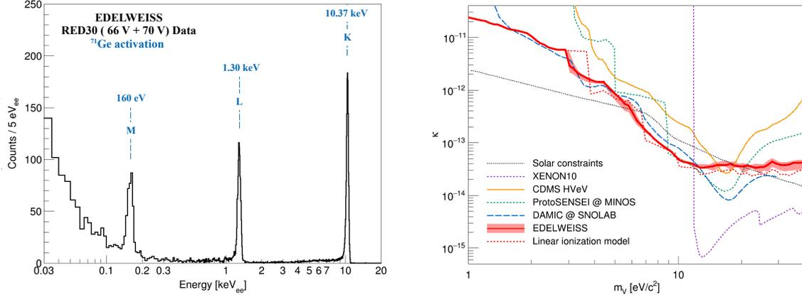
Figure 1.7: **Left:** Energy spectrum recorded with a bias of 66 V and 70 V following the  $^{71}\text{Ge}$  activation of the RED30 detector at LSM. **Right:** 90% C.L. upper limit on the kinetic mixing  $\kappa$  of a dark photon. The shaded red band and dotted red line represent alternative charge distribution models. Also shown are constraints from other direct detection experiments [137, 138, 139, 140, 141], and solar constraints [142, 143]. Figures taken from [144].
