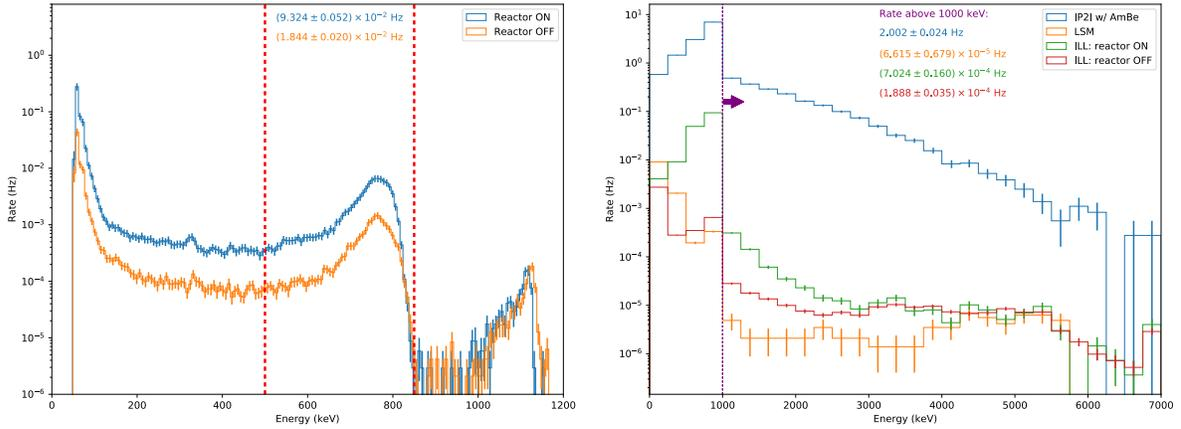
Figure 3.11: Energy distribution as observed by the ILL (**left**) and the JINR (**right**) detectors during reactor ON and OFF periods at the ILL-H7 site. For the JINR detector, we also show data taken at LSM and at IP2I with the detector exposed to an AmBe neutron source.
