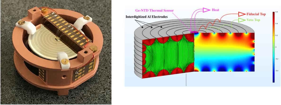
Figure 4.3: **Left:** Photo of a FID38 detector prototype where we can see the electrode rings, its NTD at the center, and the TEFLON clamps holding the crystal. **Right:** Corresponding schematic and COMSOL simulation of the FID38 detector design where we show the fiducial (green) and surface (red) volumes arising from the interleaved polarization of the veto and fiducial electrodes.
