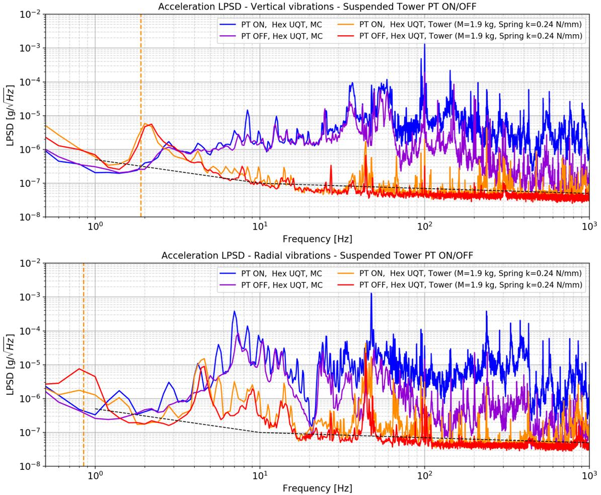
Figure 5.3: Comparison of the vertical (**top**) and radial (**bottom**) vibration levels of the MC plate and the suspended tower in both PT ON and OFF configurations. The dashed black line is the accelerometer sensitivity, and the orange vertical dashed lines represent the position of the natural frequencies of the suspended tower derived from Eqs. 5.1 and 5.2. Figures taken from [164].
