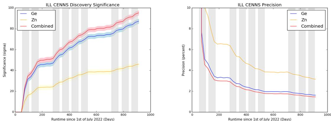
Figure 3.8: CENNS discovery significance (**left**) and precision (**right**) as a function of exposure. Median significance and precision (and 95% confidence level bands) for the discovery of CENNS using Ge (blue), Zn (yellow), and the combination of the two (red). Grey regions indicate time periods when the reactor is on.
