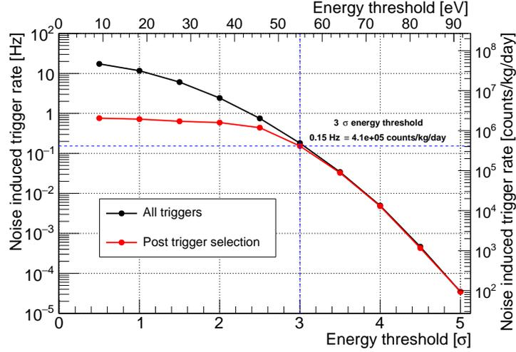
Figure 2.3: Evolution of the noise induced trigger rate (in Hz and counts/kg/day) as a function of the trigger level (in number  $n$  of  $\sigma_{OF}$  and eV), when considering (red) or not (black) the post-trigger selection.
