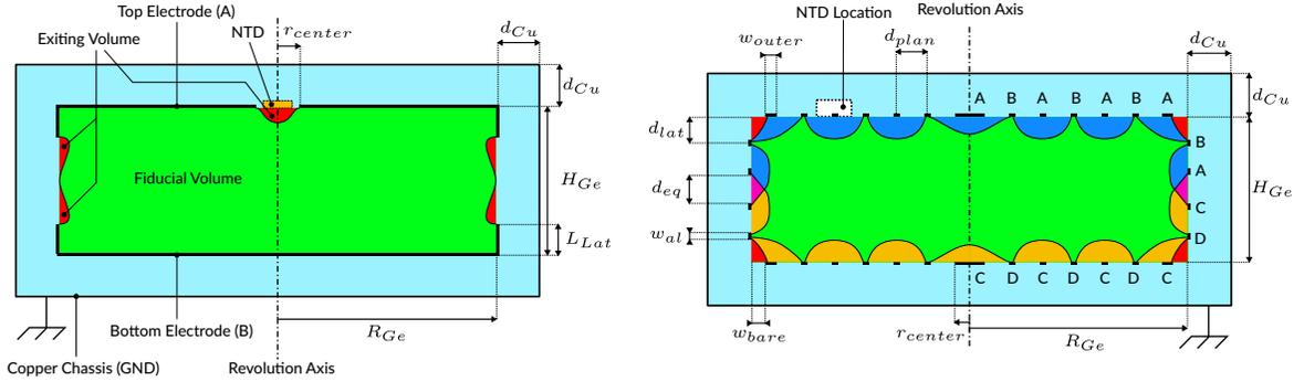
Figure 4.4: Detailed PL38 (**left**) and FID38 (**right**) detector design schematics exhibiting all of the various relevant design parameters and charge collection zones: fiducial (green), corner (red), equatorial (pink), top veto (blue), and bottom veto (yellow). The parameter values are all given in Tab. 4.2. Figure taken from [228].
