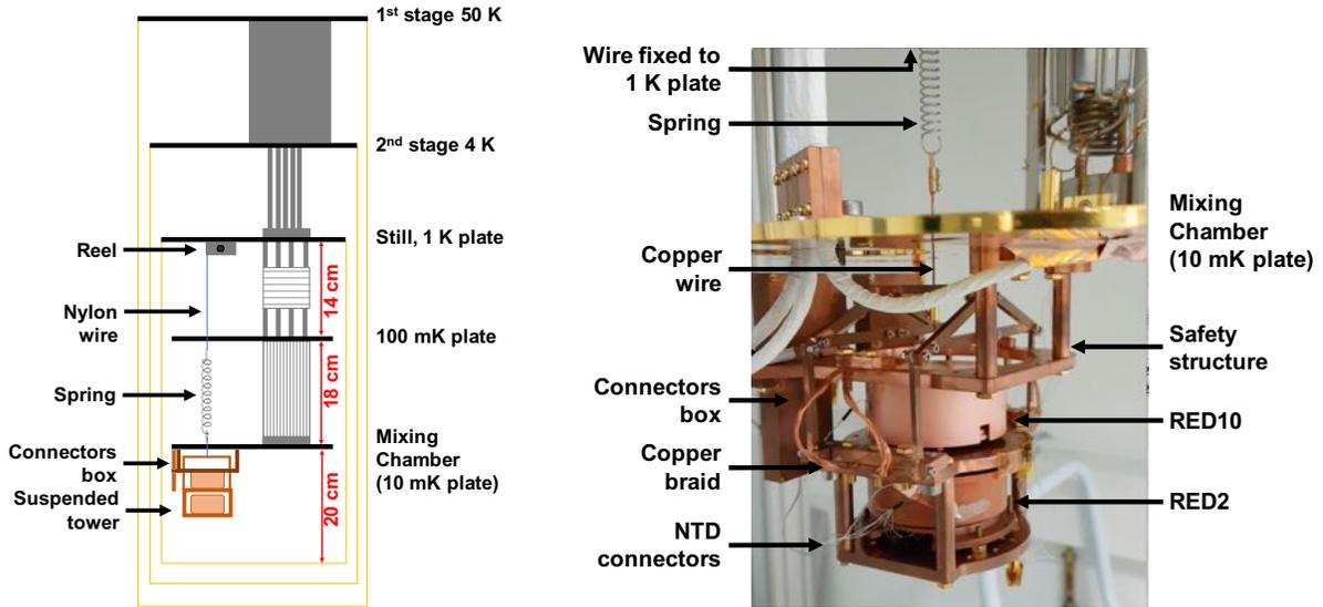
Figure 5.2: **Left:** Schematic of the suspended tower design and integration in the cryostat with a nylon wire ( $l \approx 19$  cm) and a stainless steel spring ( $k = 240$  N/m,  $l_0 = 3.4$  cm). **Right:** Suspended tower prototype hosting here two detectors (RED2 and RED10) considered for this study. Figures taken from [164].
