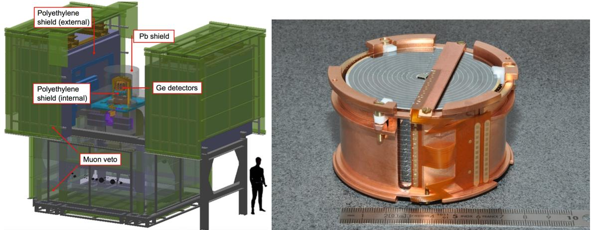
Figure 1.6: **Left:** Schematic view of the EDELWEISS-III setup showing in the center the cryostat hosting the germanium bolometers, surrounded by passive lead (Pb) and polyethylene shields and an active muon veto in order to protect the detectors from various backgrounds. **Right:** Photo of an 860-g FID detector with concentric ring electrodes covering the entire crystal surface and embedded in its copper casing held by Teflon clamps. Figures taken from [80].
