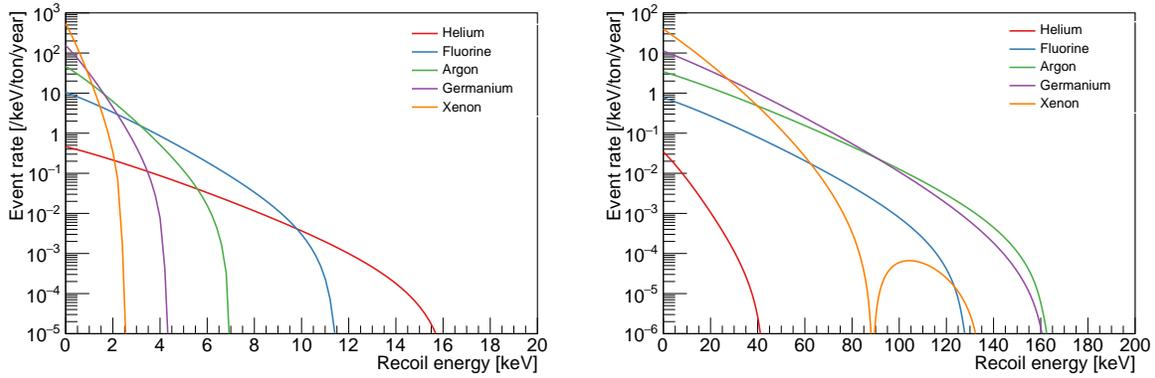
Figure 1.1: Differential event rate for various detector target materials: Helium (red), Fluorine (blue), Argon (green), Germanium (purple), and Xenon (orange), for a 5 GeV/c<sup>2</sup> (left) and a 50 GeV/c<sup>2</sup> (right) WIMP mass. The calculations have been done considering the standard halo model parameters and a SI WIMP-nucleon cross section of 10<sup>-45</sup> cm<sup>2</sup>.
