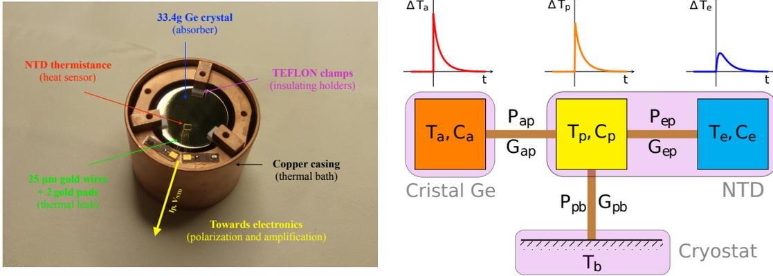
Figure 4.1: **Left:** Picture of the RED20 detector prototype where all the relevant components related to its thermal modelization are labeled. **Right:** Simplified block diagram of the thermal modelization of the RED20 detector (*Courtesy of D. Misiak*).
