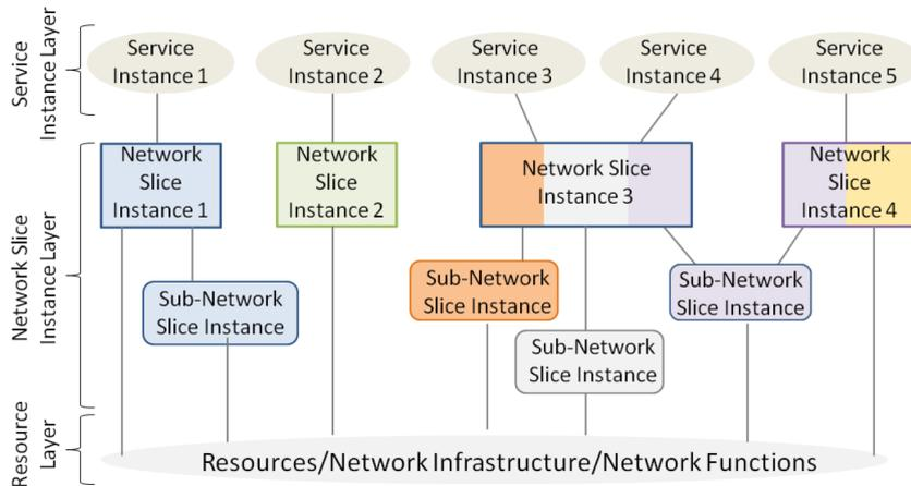
Figure 2.4 – Network slicing layers
