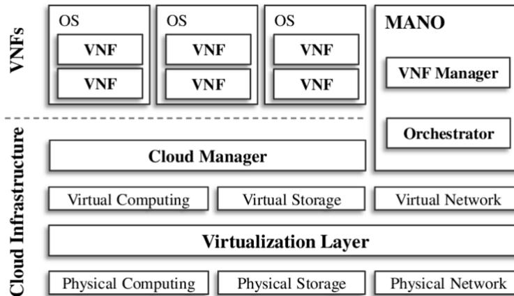
Figure 2.6 – Architecture for NFV
