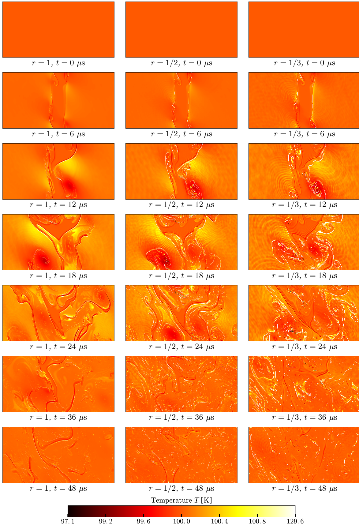
Figure 11.20: Evolution in time of the temperature profiles for two-dimensional periodic Nitrogen liquid jets in their vapor. Three cases have been carried out for Re = 1470 ( We = 4150 ) with the reference thickening factor F = 1000 and three different spatial resolutions (left: reference r = 1 , center: coarse r = 1/2 , right: very coarse r = 1/3 )
