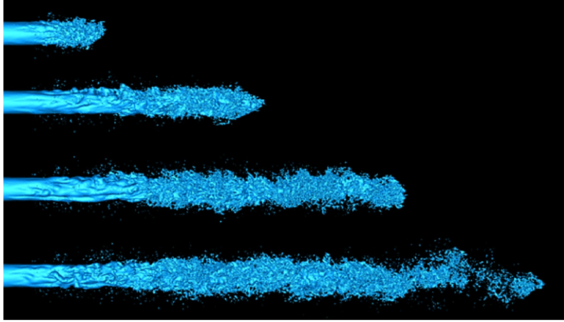
Figure 3.19: Simulation of the turbulent atomization of a liquid Diesel with the Accurate Conservative Level-Set method, from Desjardins et al. (2008)
