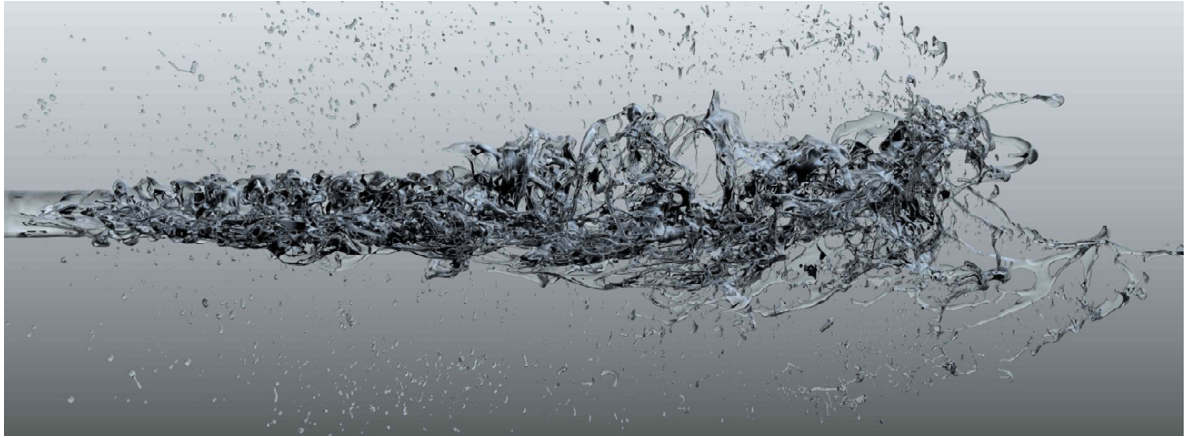
Figure 3.9: Snapshot of the atomization of a round water jet in a quiescent air from Le Chenadec and Pitsch (2013)
