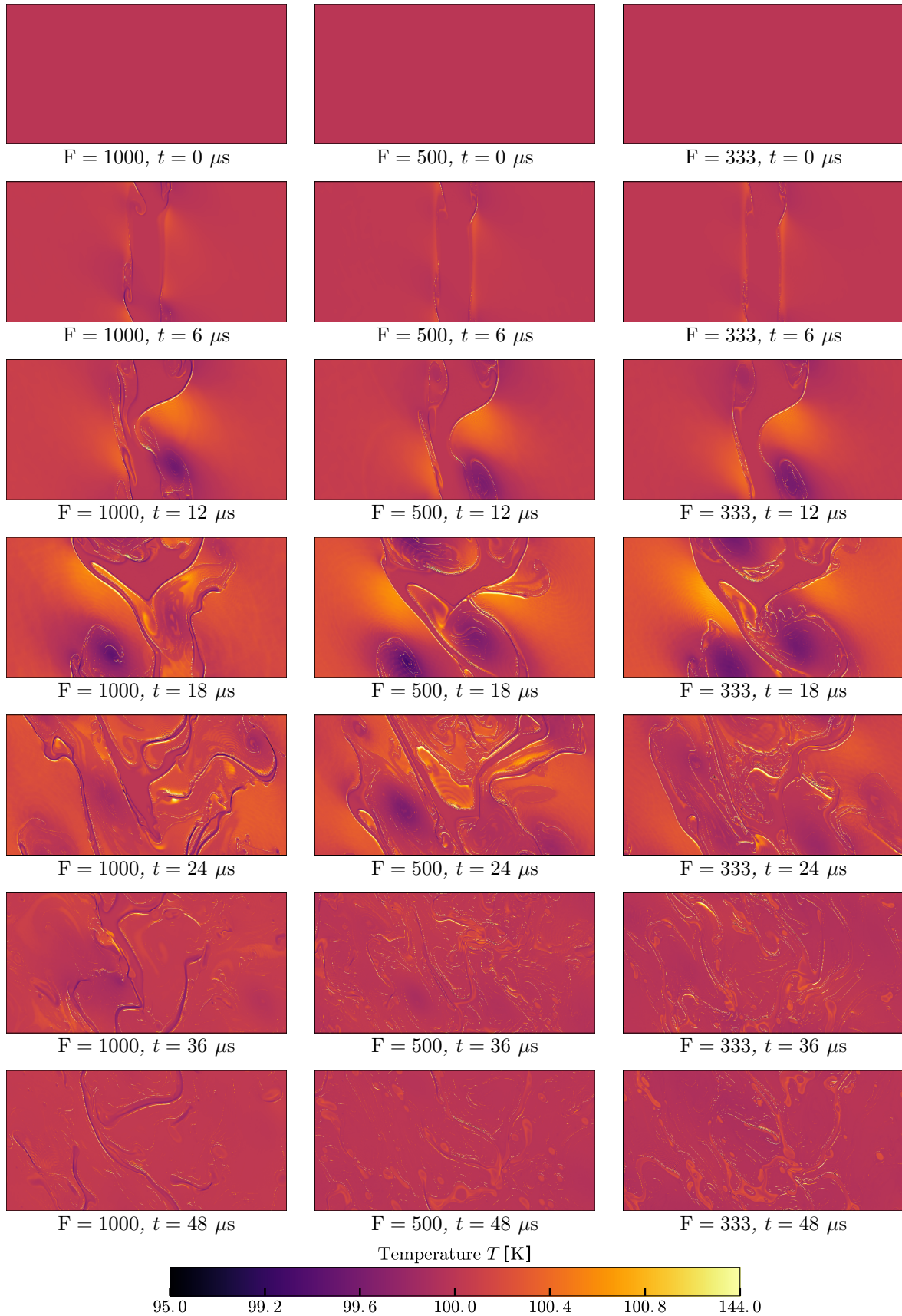
Figure 11.26: Evolution in time of the temperature profiles for two-dimensional periodic Nitrogen liquid jets in their vapor. Three cases have been carried out at Re = 1470 (4150) with the reference spatial resolution and three different thickening factors (left: large F = 1000 , center: medium F = 500 , right: low F = 333 )
