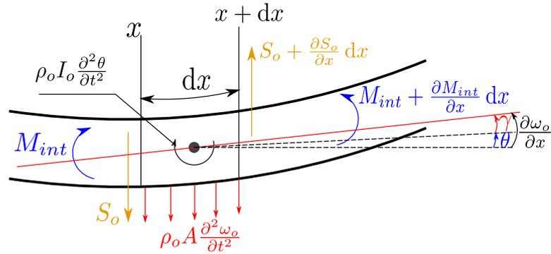
Figure II.14 – Force diagram of the Timoshenko beam.
