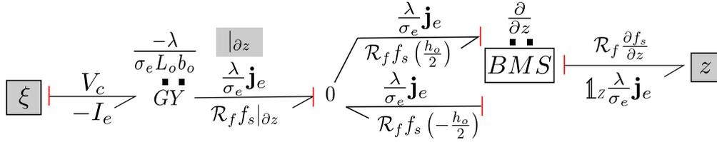
Figure II.18 – Bond graph of the coupling between electrical system and electro-stress diffusion system.
