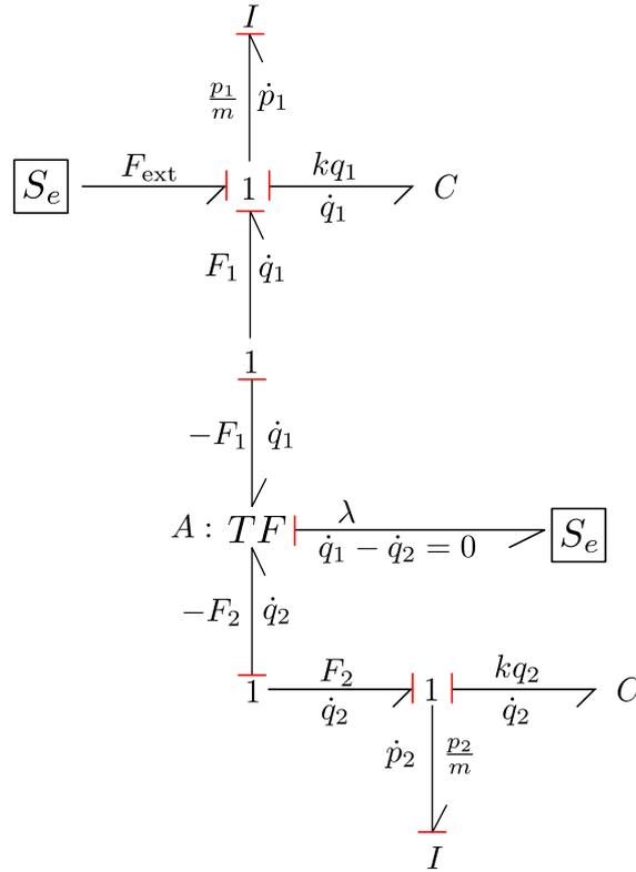
Figure I.11 – Bond Graph of two glued mass-spring systems.
