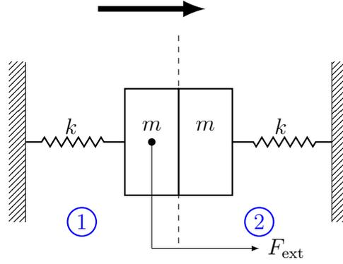
Figure I.9 – Schema of two glued mass-spring systems.
