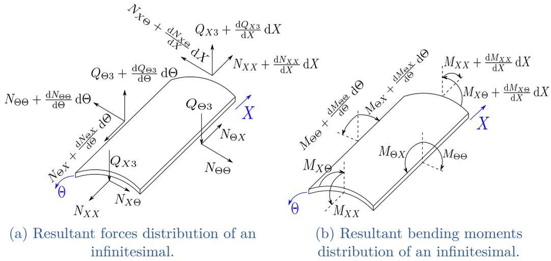
Figure II.23 – Resultant forces and bending moments diagram.
