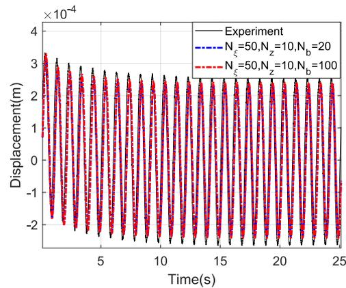
Figure III.16 – Tip deflection of IPMC strip with a sinusoidal input voltage.
