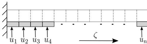
Figure IV.3 – Clamped-free vibrating string with fully-actuated case.
