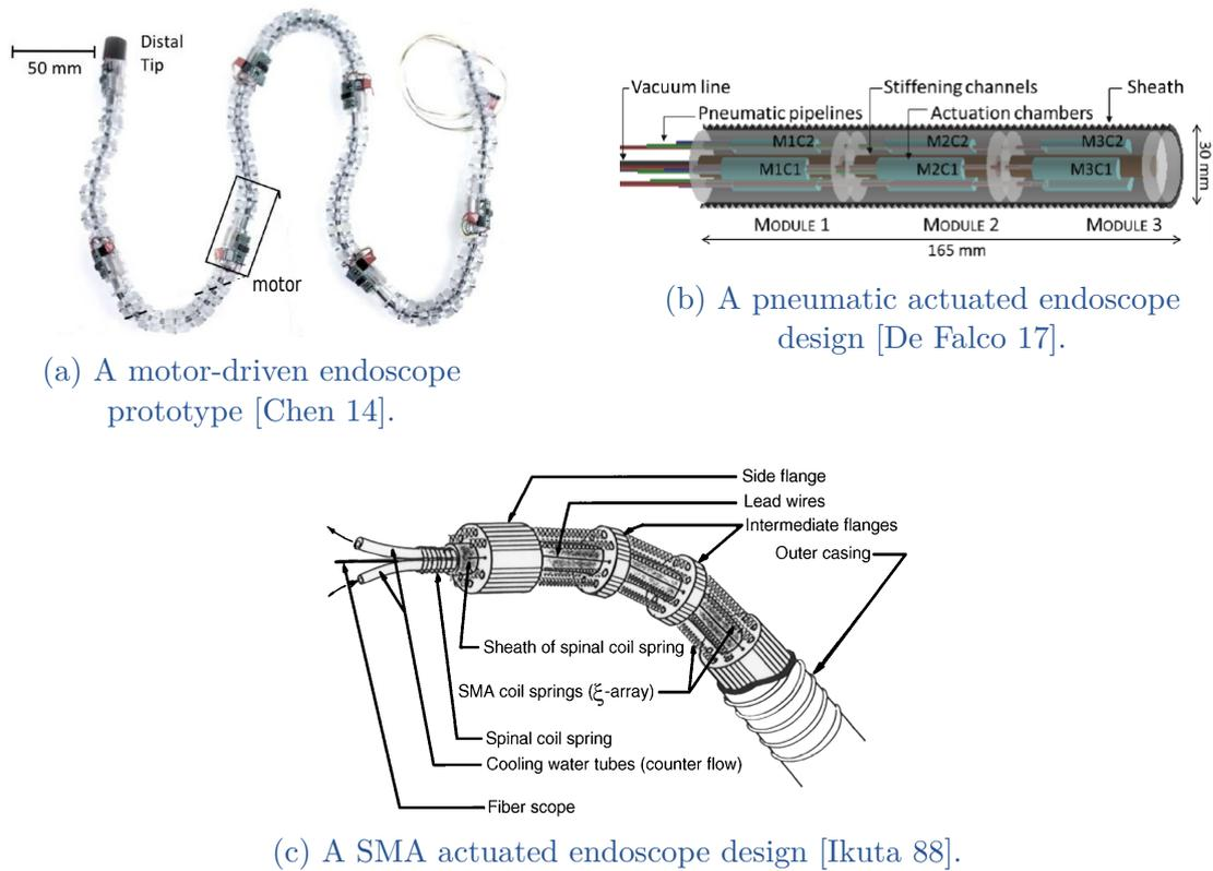
Figure I.5 – Various actuation principles of endoscopes.
