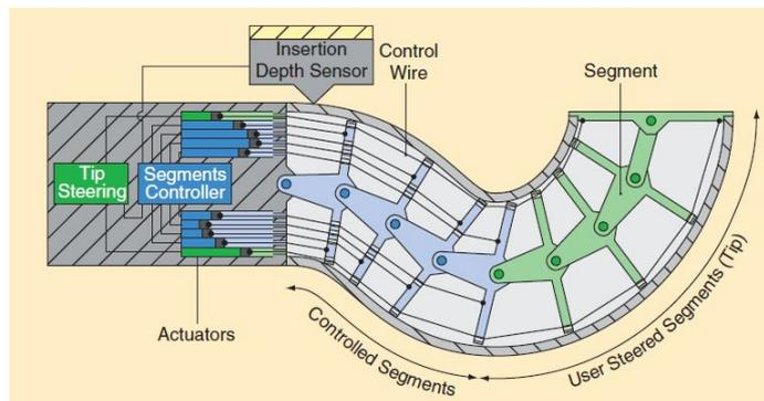
Figure I.4 – Wire-driven push-pull manipulation of flexible endoscopes [Loeve 10].
