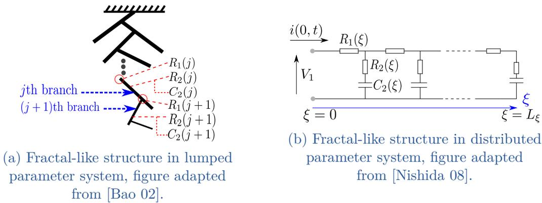
Figure II.8 – Models of IPMC electrodes interface.
