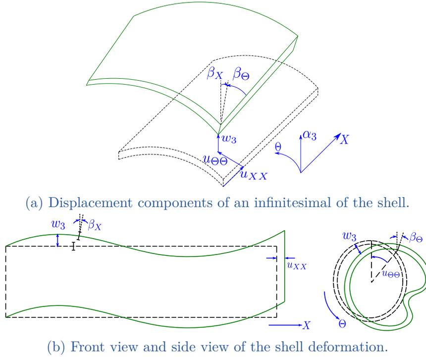
Figure II.22 – Deformation of the shell model.
