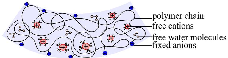
Figure II.11 – Solid and liquid phases of the gel.
