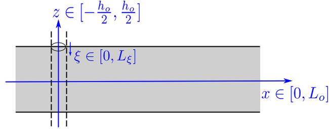
Figure II.5 – Coordinates representation of the IPMC actuator.
