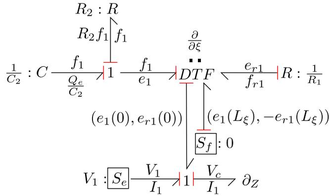
Figure II.9 – Bond Graph of the electrical system dynamics.
