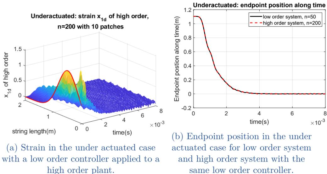
Figure IV.13 – Closed loop evolution of the strain of the high order system, and comparison of the endpoint position of the low order and high order systems using the same controller.
