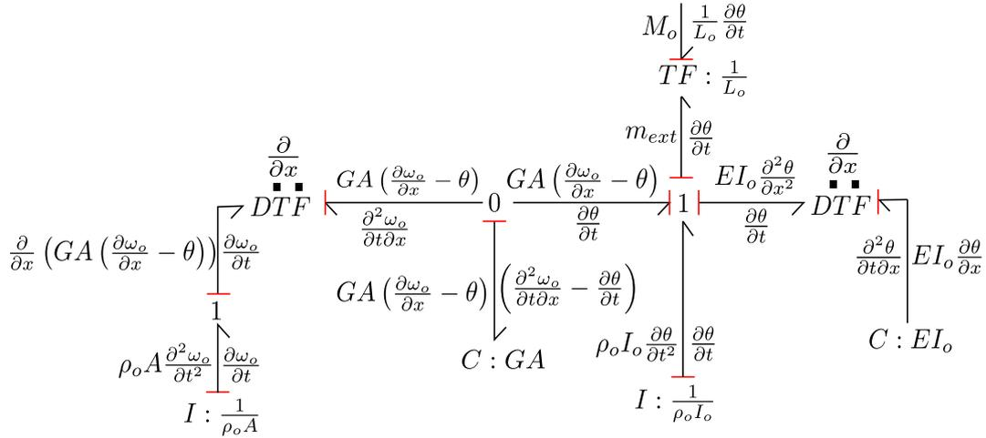
Figure II.15 – Bond Graph of the mechanical system dynamics.
