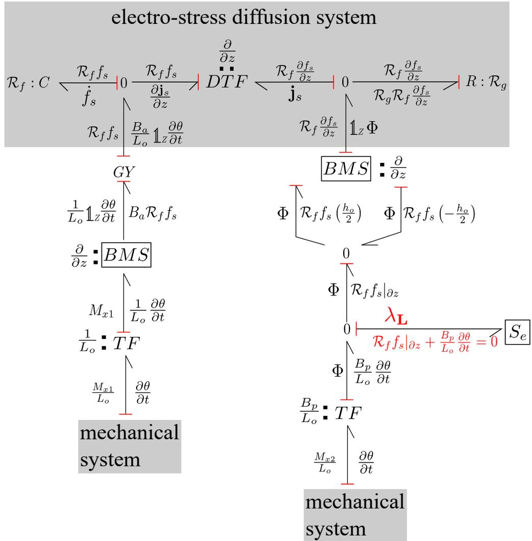
Figure II.19 – Bond graph of the coupling between the electro-stress diffusion system and the mechanical system, through  $\frac{M_{x1}}{L_o}(x, t)$  (left column),  $\frac{M_{x2}}{L_o}(x, t)$  (right column) and  $\frac{\partial \theta}{\partial t}(x, t)$ .
