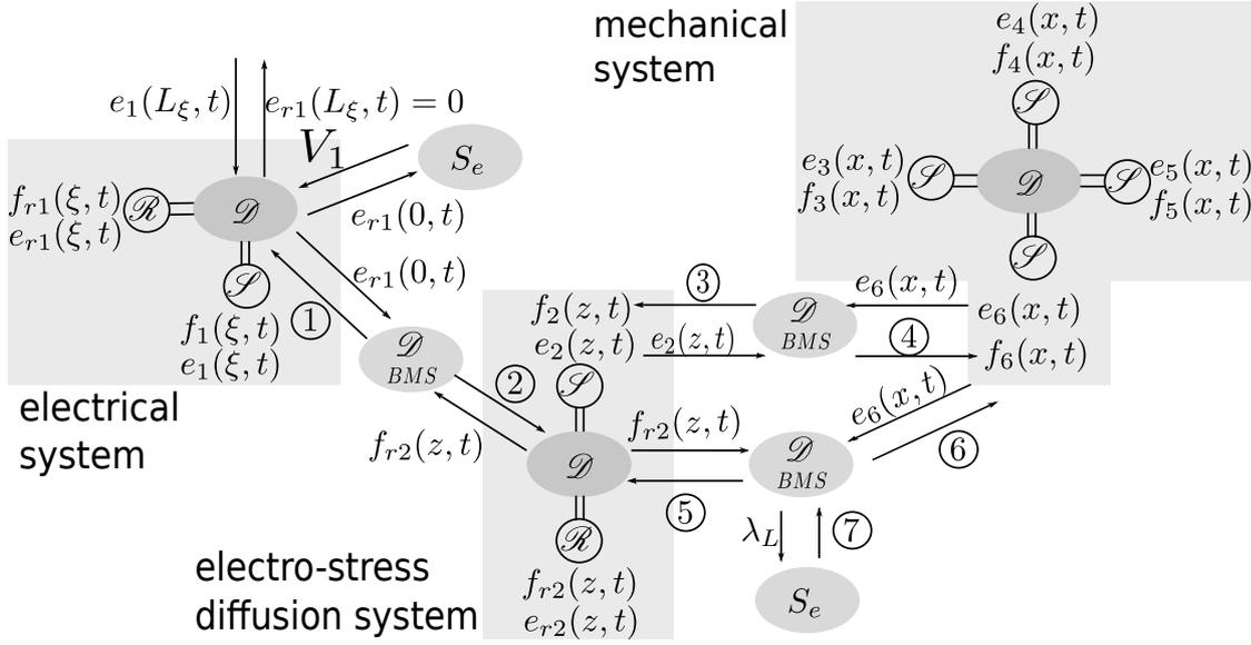
Figure II.20 – Schema of the overall IPMC actuator model.
