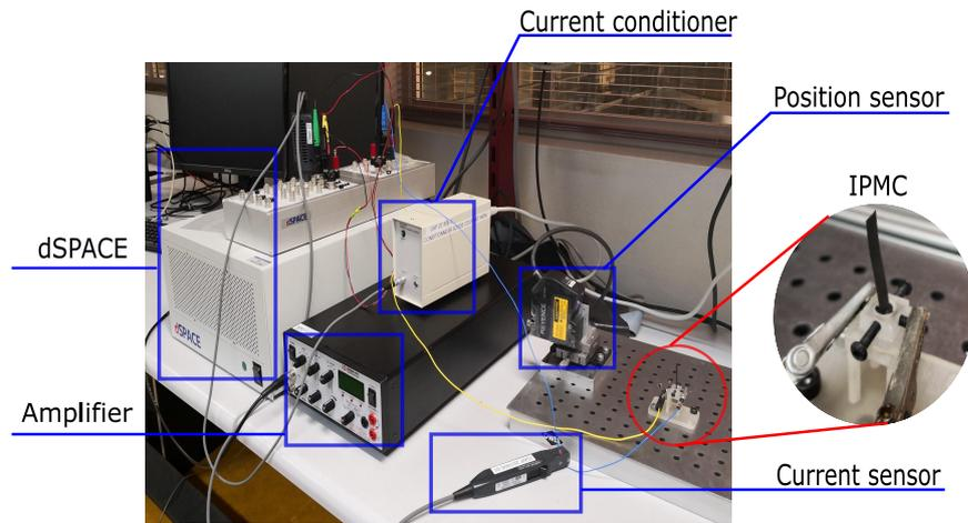
Figure III.10 – Experimental setup of the IPMC actuator.
