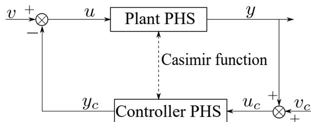
Figure I.12 – Schema bloc of CbI for PHS.
