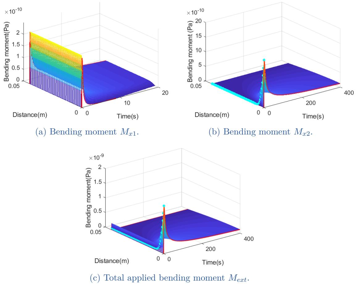
Figure III.15 – Simulation results for  $M_{x1}$ ,  $M_{x2}$  and  $M_{ext}$  along x-axis and the time ( $N_\xi = 50$ ,  $N_z = 10$  and  $N_b = 100$ ).
