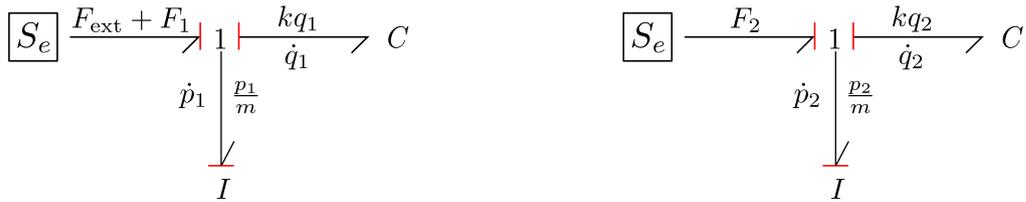
Figure I.10 – Bond Graph of two separate mass-spring systems.
