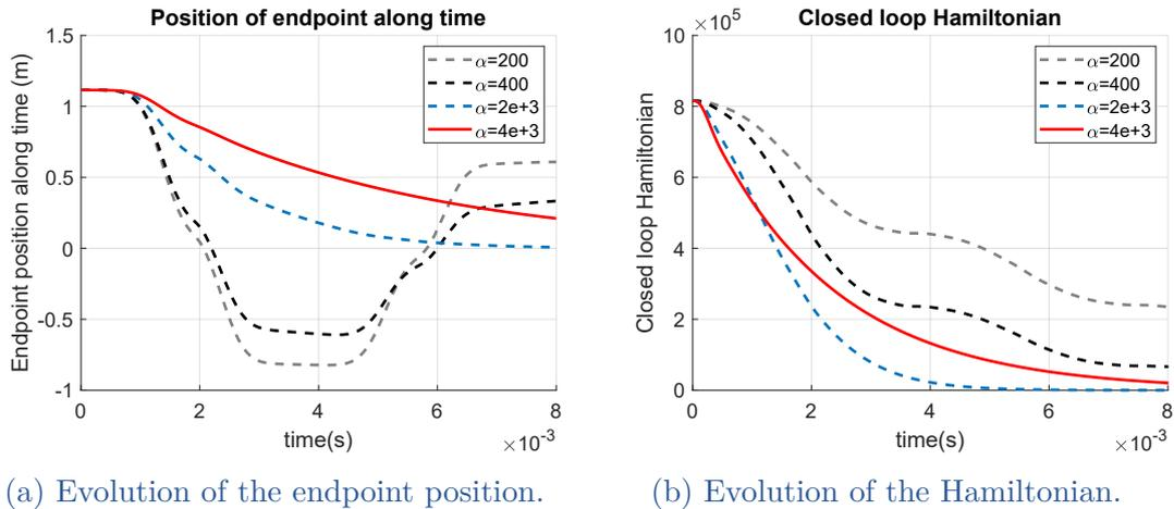
Figure IV.6 – Closed loop simulation in the fully-actuated case with pure damping injection and different damping coefficients  $\alpha$ .
