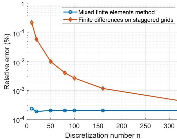
Figure III.6 – Relative approximation error of the mixed finite element method and of the finite difference method on staggered grids with different discretized number  $n = 10, 20, 50, 80, 100, 160, 320$ .
