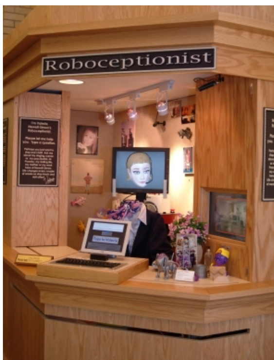
Figure 4.6 – The permanent installation of the receptionist Valerie (Gockley et al., 2005). It was built on a mobile base with a moving flat-panel monitor mounted on top, displaying a graphical expressive human-like face.
