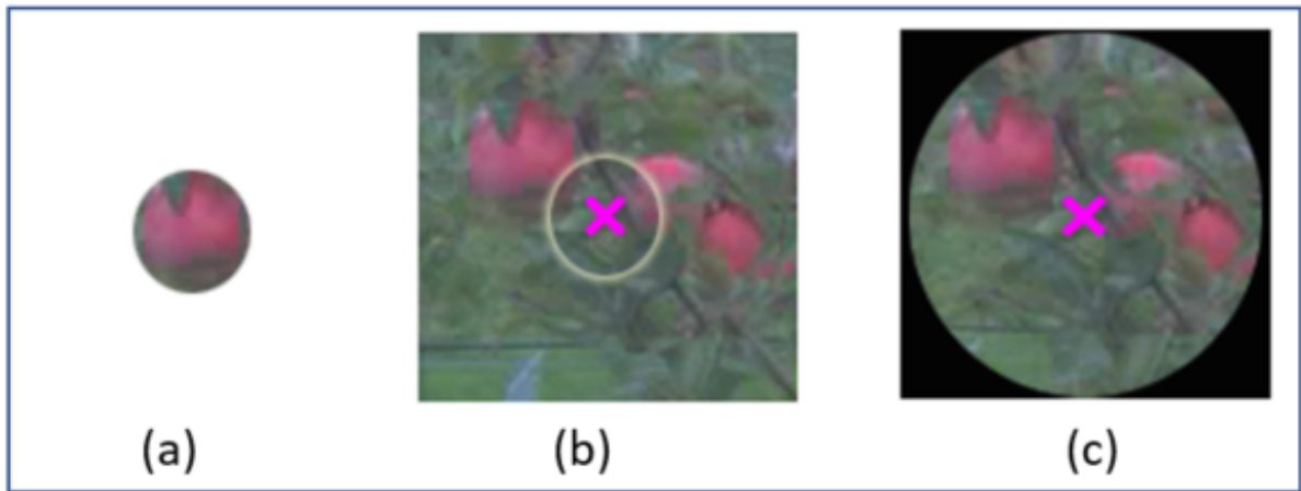
Figure 3.11 – Construction of attention areas. (a) The average diameter of an average apple is 30 pixels in our dataset; (b) Cross indicates the center of the gaze of the annotator. There is a shift error from the apple of (a). The maximum distance of the gazing point with the center of the closest object is found at 169 pixels ; (c) Chosen attention area with a size of 180 \times 180 (pixels).
