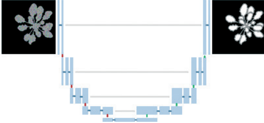
Figure 3.15 – U-Net architecture. Each blue box corresponds to a multi-channel feature map. The input image has 128x128 pixels, the output of the model is a three-channel binary image: mask without contours, leaf contours, and background.
