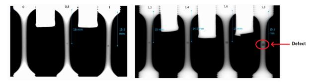
Figure 2.4 – Coupons incorporating spherical defects of size varying from 0 mm (on the left) to 1.8 mm (on the right)
