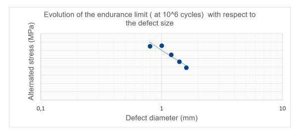
Figure 2.5 – Mean allowable stress with respect to the defect size
