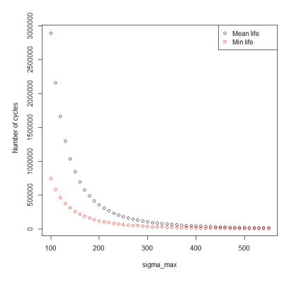
Figure 3.5 – Evolution of the mean and minimum propagation time  $N_p$  with respect to the maximum loading  $\sigma_{\rm max}$
