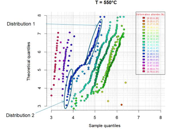
Figure 3.1 – Quantile-quantile Gaussian plot of the logarithm of the numbers of cycles to failure for different levels of strain, nickel based material,  $T = 550^{\circ}C$
