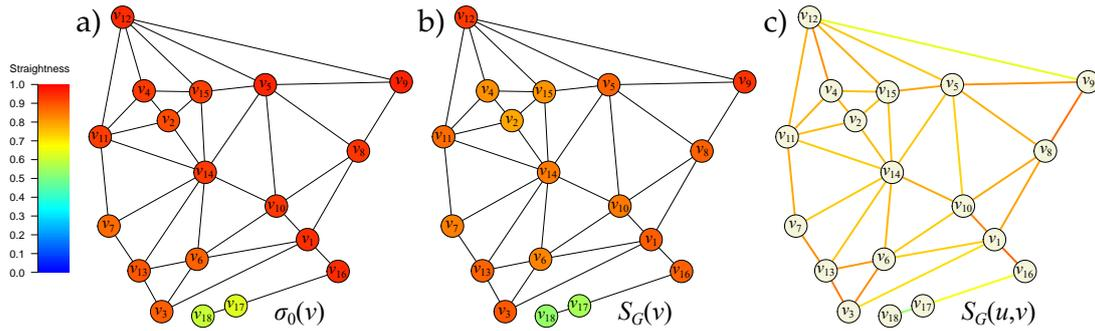
**Figure 6.12:** Straightness obtained for a random spatial graph: average vertex-to-vertex Straightness  $\sigma_0(v)$  (a); average continuous Straightness for each vertex  $S_G(v)$  (b) and edge  $S_G(u, v)$  (c).
