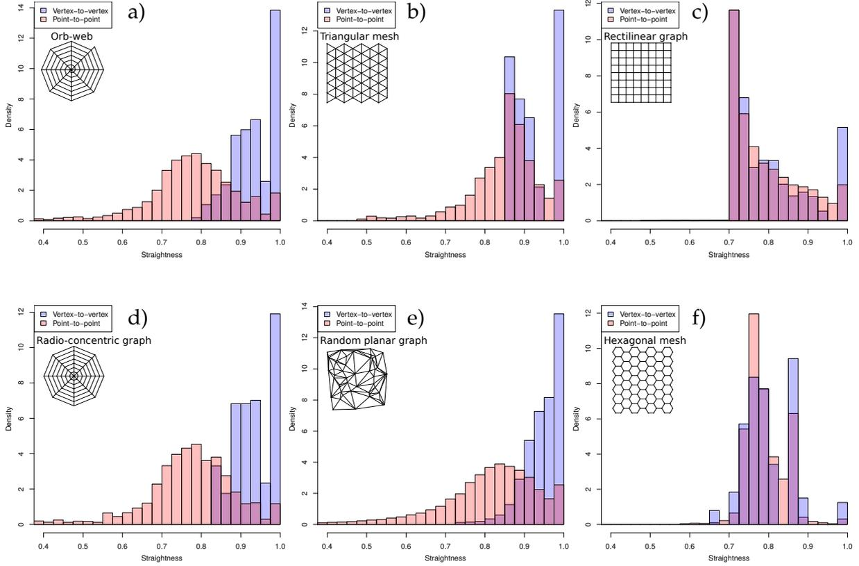
**Figure 6.8:** Distribution of the Straightness over each pair of vertices (blue) and points (red) in 6 types of spatial networks: orb-web (a); triangular mesh (b); rectilinear (c); radio-concentric (d); random planar (e); and hexagonal mesh (f).
