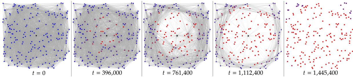
**Figure 4.9:** Example of the evolution of a Wireless Sensor Network. The sink is represented as a black square, whereas the rest of the vertices are sensors. Their color indicate their battery level, from full (blue) to empty (red). Dead sensors are represented by squares and alive ones by circles. Edges represent the possibility for one vertex to communicate with another.
