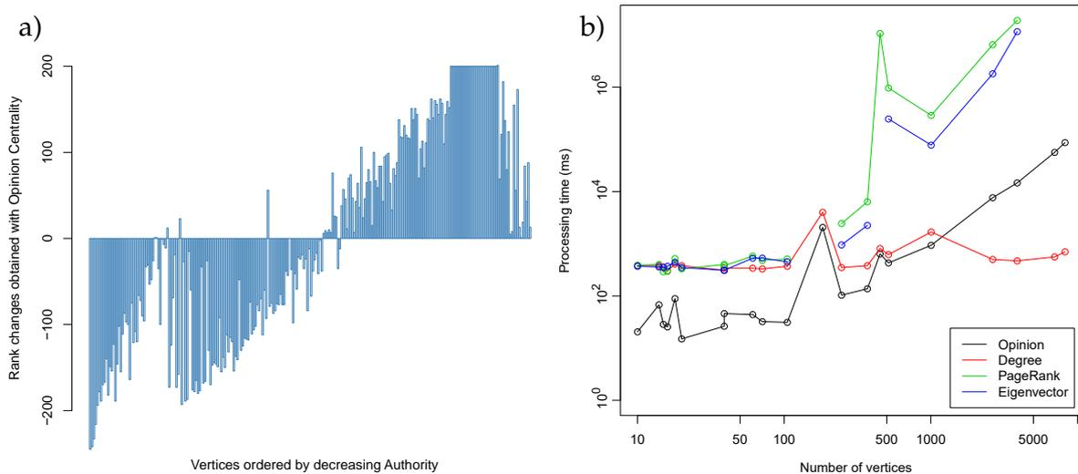
**Figure 8.3:** a) Rank difference between the Opinion centrality and the Authority measure, for each individual vertex in the CKM Physicians network. Each bar corresponds to a vertex, and its height matches the rank difference. b) Processing times of the main considered measures, as functions of the numbers of vertices.
