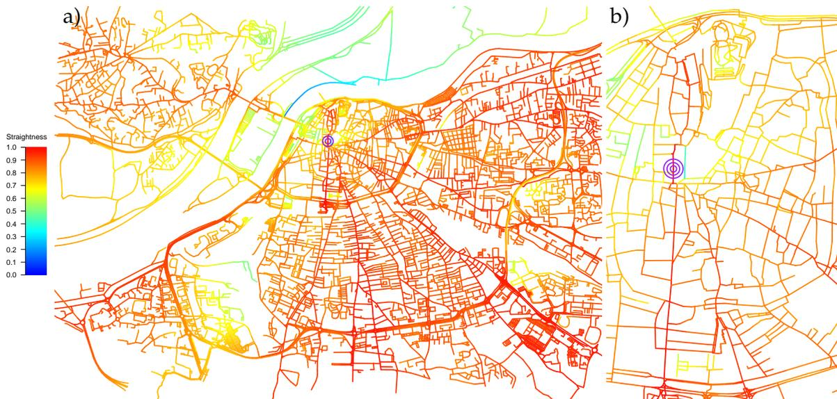
**Figure 6.13:** Straightness obtained for the city of Avignon, France: whole city (a) and city center (b). The color gradient corresponds to  $S_{uv}(r)$ , the average Straightness between a fixed vertex corresponding to the city hall (represented in purple) and each edge of the graph. Vertices are not represented to ease distinguishing the edges color.
