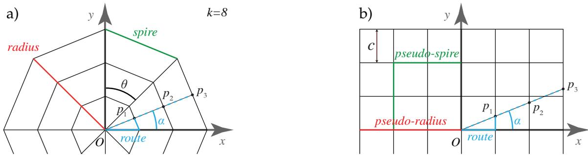
**Figure 6.6:** Terminology and notations used to describe the radio-concentric (a) and rectilinear (b) networks.
