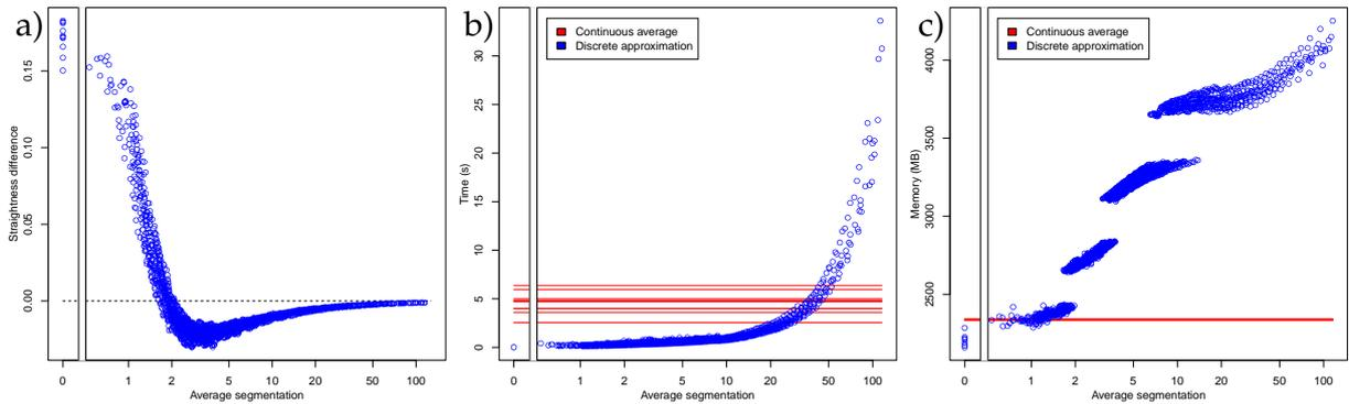
**Figure 6.11:** Results obtained on random planar graphs, as functions of the average edge segmentation  $\beta$ . (a) Difference between the discrete approximation and the continuous Straightness ( $\sigma_\beta(G) - S_G(G)$ ). (b) Processing time and (c) memory usage required by the continuous average Straightness  $S_G(G)$  (red) and its discrete approximation  $\sigma_\beta(G)$  (blue).
