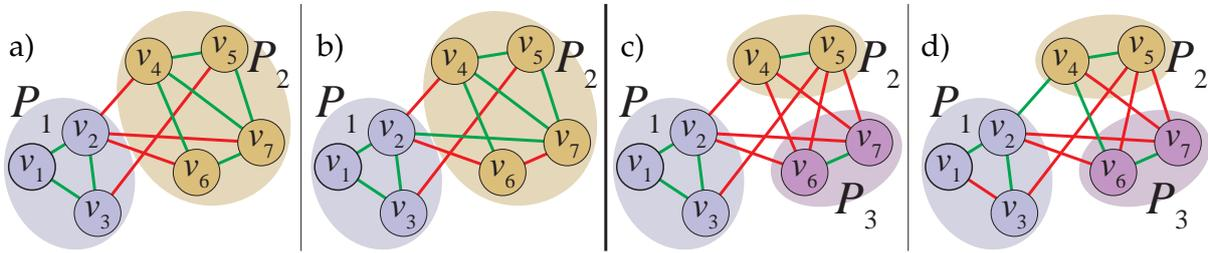
**Figure 7.3:** Examples of strongly and weakly balanced and imbalanced graphs: (a) strongly and weakly balanced ( $I(G, \mathcal{P}) = 0$ ); (b) strongly and weakly imbalanced ( $I(G, \mathcal{P}) = 2$ ); (c) strongly imbalanced but weakly balanced ( $I(G, \mathcal{P}) = 0$ ); (d) strongly and weakly imbalanced ( $I(G, \mathcal{P}) = 3$ ).
