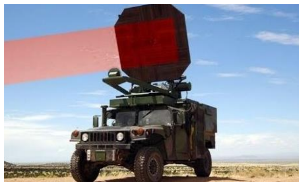
Figure I. 10 : Active Denial System à 95 GHz [21]
