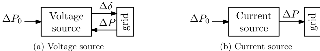
Figure D.1 – Generic representation of the simplified models of voltage and current sources connected to the grid.
