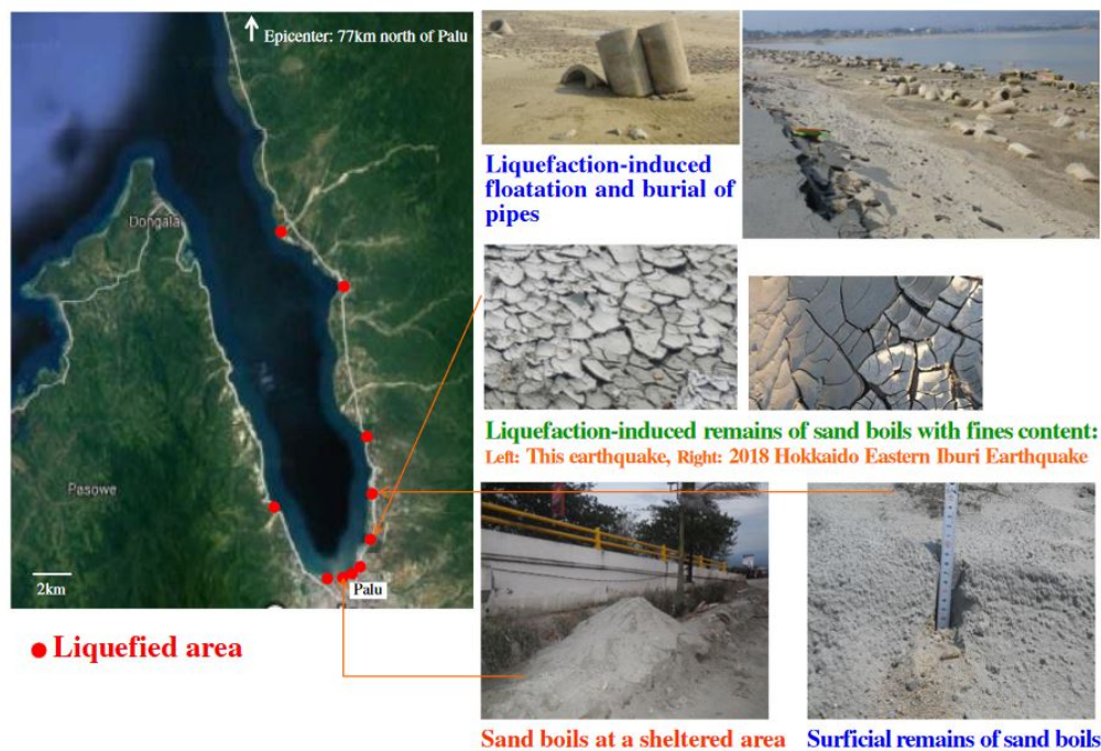
Figure 2.6: Evidence of extensive coastal liquefaction during the 2018 Indonesia Sulawesi earthquake (Sassa and Takagawa, 2019).
