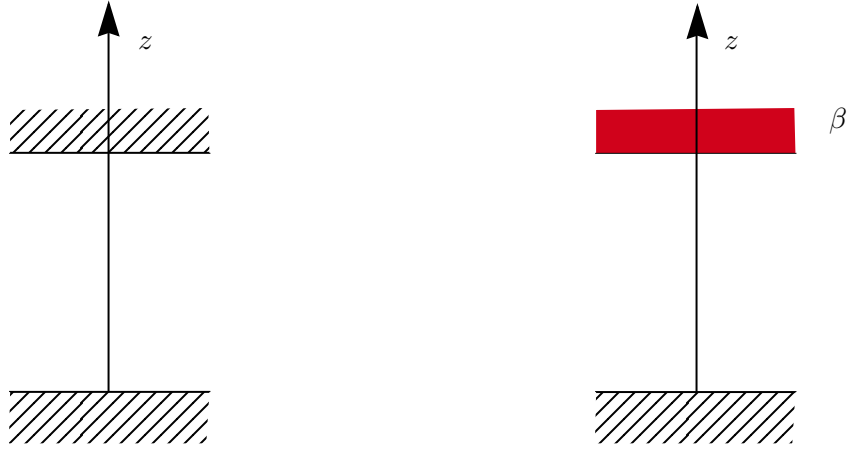
Figure 3.2: Sketches of a rigid duct case (left) and a lined duct case (right).
