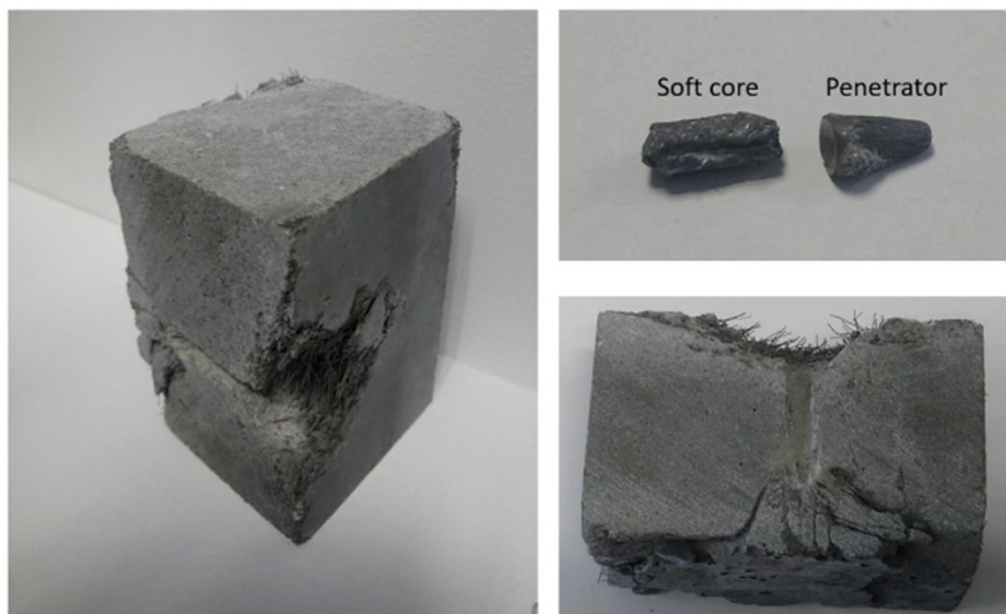
Fig 4.1 – Views of the impacted target of Ductal® B-2% (60x60x95 mm) and recovered parts of the bullet after impact: penetrator 4.8 mm in diameter, 10 mm in length, soft core 4.1 mm in diameter and 8 mm in length (final dimensions)
