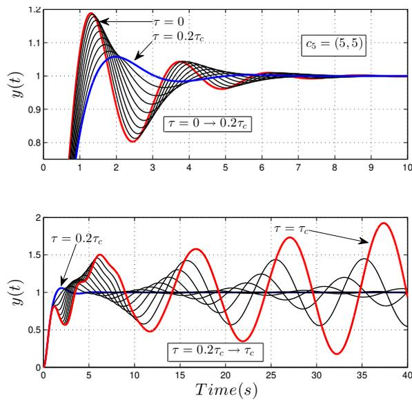
Figure 2.11:  $P\delta I$  Controller: Closed-Loop System Response with  $\tau \in (0, \tau_c)$
