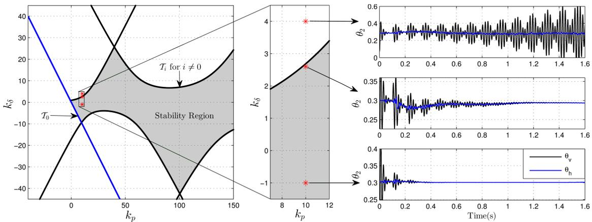
Figure 3.2: Stability regions vs Experimental Behaviour for the Second Joint
