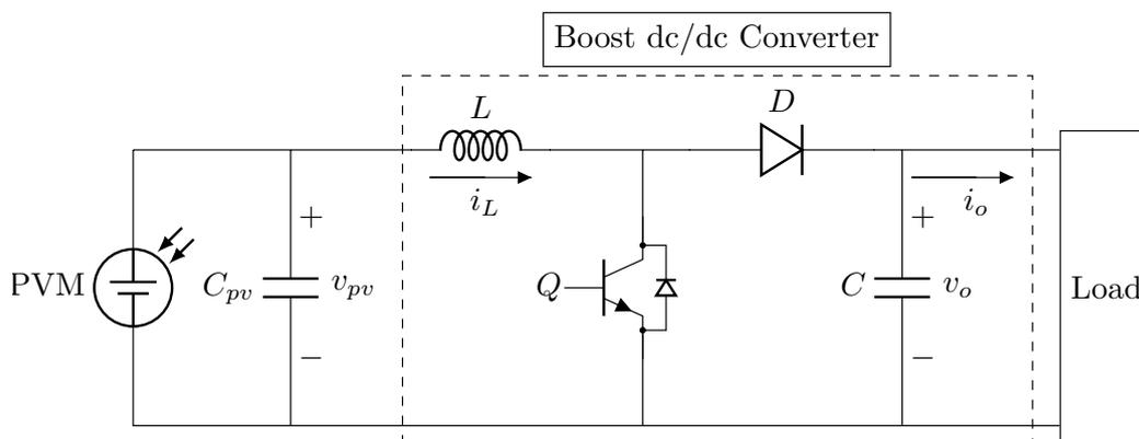
Figure 4.1: MPPT System Considering a Boost DC/DC Converter
