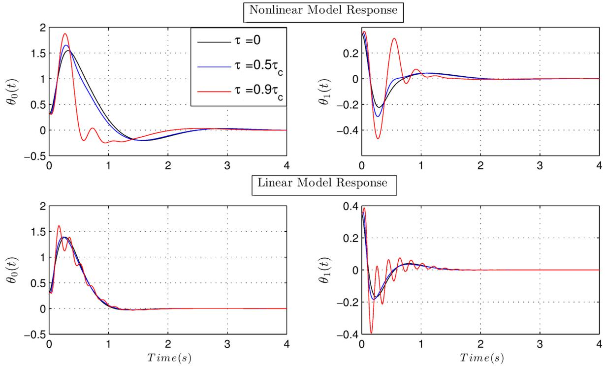
Figure 3.17: Closed-Loop System Response Under Different Delay Values.
