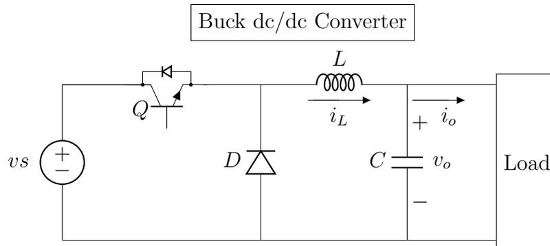
Figure 3.10: Topology of the Buck DC/DC Converter [72].
