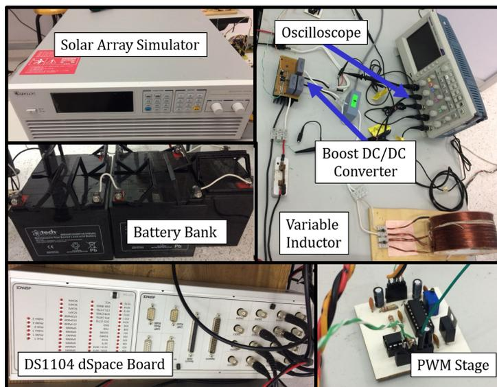
Figure 4.2: Experimental Test Bench - Main Components
