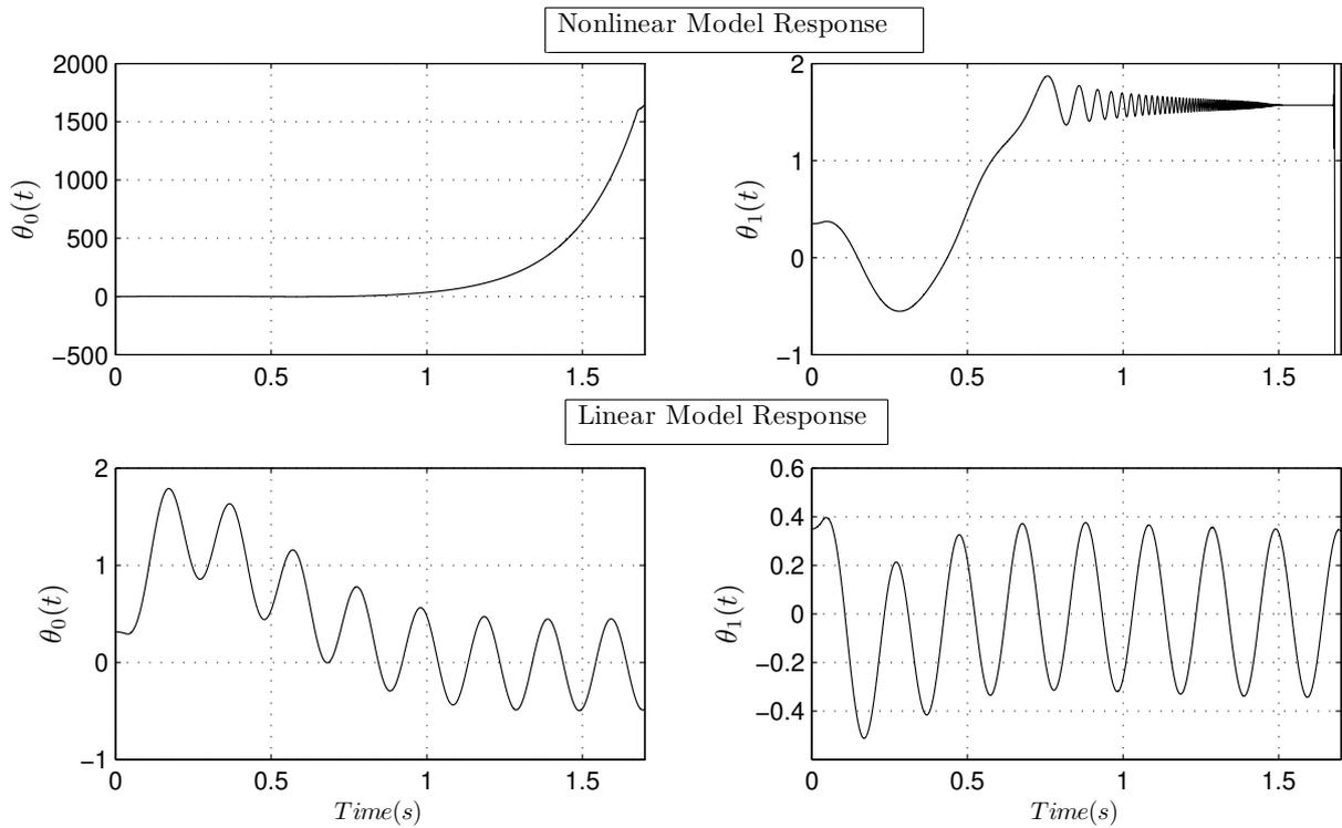
Figure 3.18: Closed-Loop System Unstable Response Under a Critical Delay.
