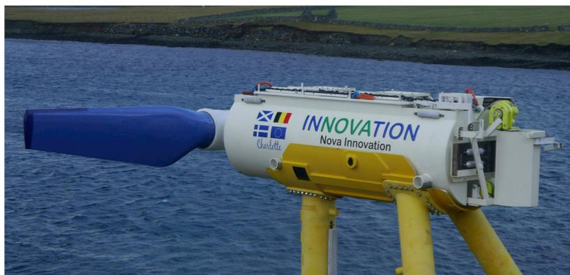
FIGURE 2.22: D2T2 tidal stream turbine (©Nova Innovation) [22].
