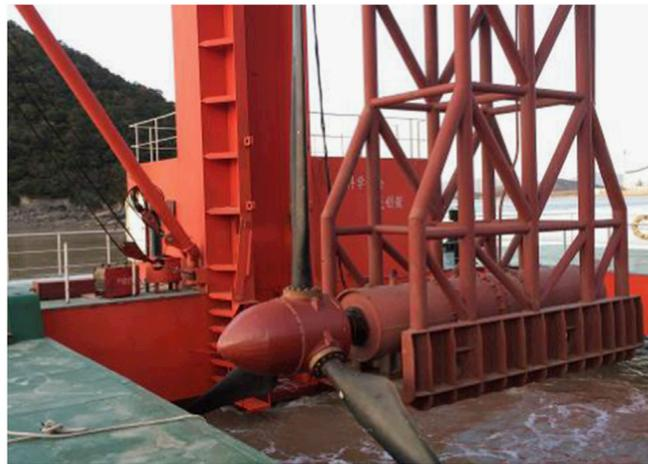
FIGURE 2.16: Small scale Multibrid tidal stream turbine [16].
