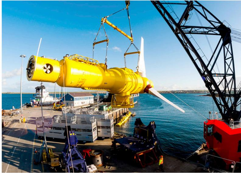
FIGURE 2.2: GE/Alstom geared tidal stream turbine [1].
