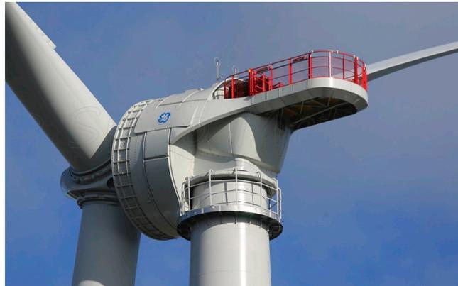
FIGURE 2.9: GE/Alstom 6 MW Haliade 150 offshore wind turbine [9].
