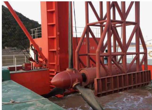
FIGURE 2.16: Small scale Multibrid tidal stream turbine [16].
