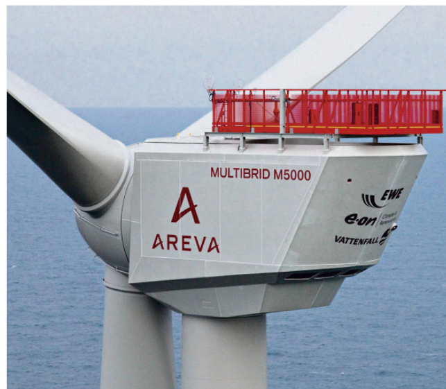
FIGURE 2.14: View of the Areva Multibrid M5000 wind turbine with 2-stage gearbox (Areva) [15].
