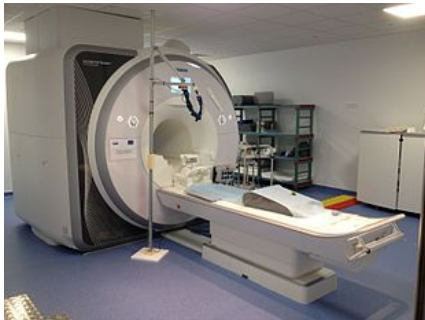
Figure 1.2-4 – MRI scanner of 3T . Example of a 3T MRI system installed at Neurospin (CEA Saclay, France) to perform structural or functional neuroimaging.
