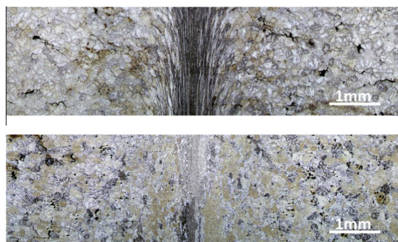
Fig. 1. Optical micrographs of the linear friction weld (interface plane is vertical in the centre of the micrograph) in the as-welded state (top) and after the interdiffusion heat treatment (bottom).
