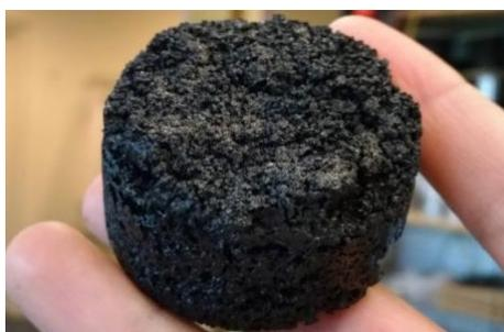
**Figure 7.13** Asphalt-like material obtained by humins-lignin (75-25 %) composite.
