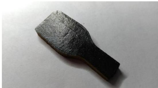
**Figure 7.12** Humins-lignin (40 % wt.) composites – Black Wood.
