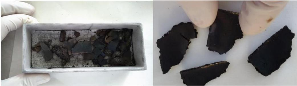
**Figure 7.8** Carbon-based conducting material with no porosity produced with a carbonization of crude humins at 900 °C using 1 °C·min<sup>-1</sup> ramp.
