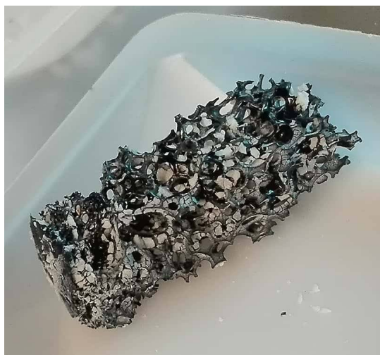
Figure 6.3 Picture of alumina deposition on a humins foam with an alkaline pretreatment.
