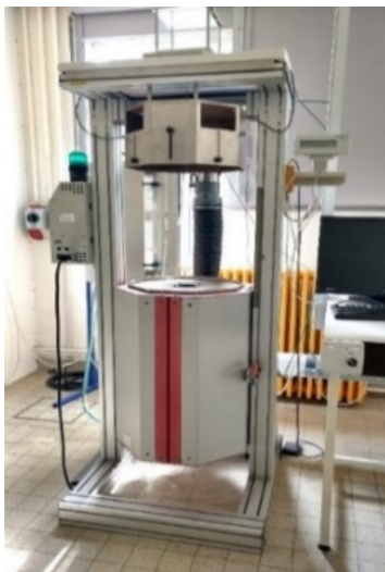
Figure 4.7 Large scale simultaneous TGA-DTA instrument built at INERIS.
