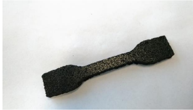
Figure 7.11 Dog-bone sample of humins-chitosan (85-15%).
