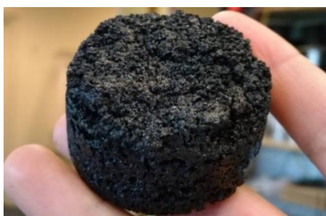
Figure 7.13 Asphalt-like material obtained by humins-lignin (75-25 %) composite.
