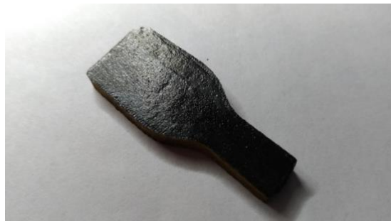
Figure 7.12 Humins-lignin (40 % wt.) composites – Black Wood.
