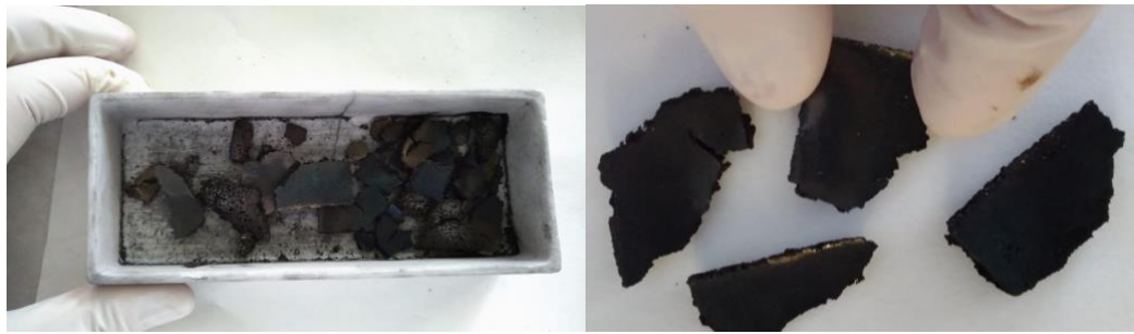
Figure 7.8 Carbon-based conducting material with no porosity produced with a carbonization of crude humins at 900 °C using 1 °C·min -1 ramp.
