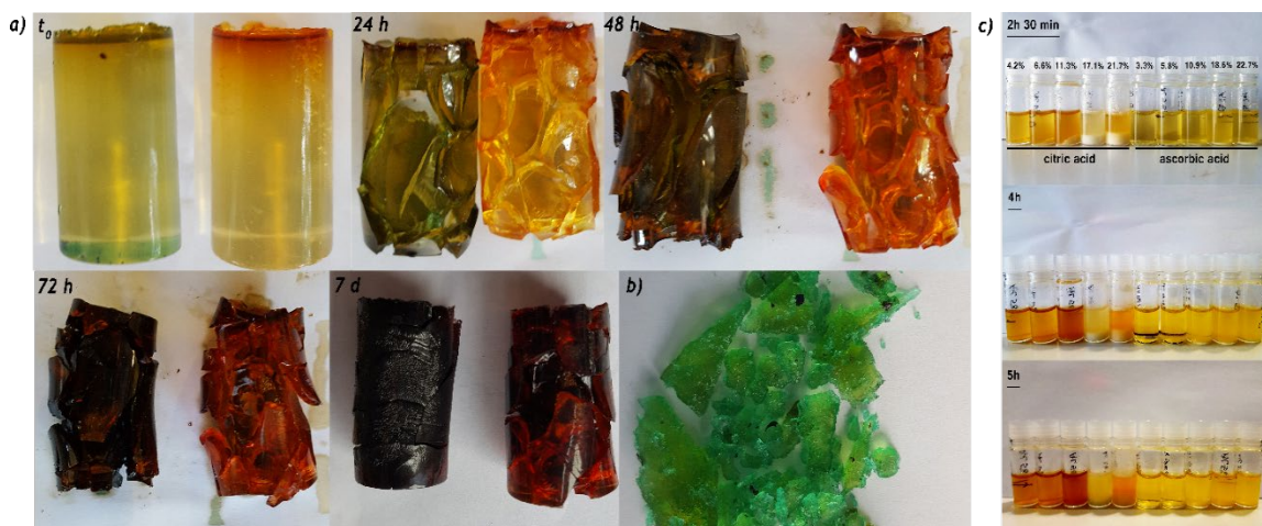
Figure 3.3 Oxidation of dopamine-functionalized PAAm hydrogels with (right) or without (left) 5% ascorbic acid, when left in open contact with air in a controlled moisture environment (a). Oxidation of a dopamine-functionalized hydrogel after 21 days in a closed vial (b). Oxidation of dopamine-functionalized hydrogel over time with increasing concentrations of citric acid or ascorbic acid (c).
