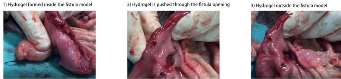
Figure 4.5 Ex-vivo test of a hybrid alginate/PAAm hydrogel for fistula closure on a fistula model prepared by anastomosis of a section of small bowel on the stomach wall.
