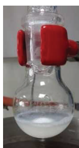
Figure 63 The initially transparent nanoparticle-BPPEG mixture becomes turbid at the cloud point of BPPEG.
