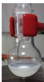
Figure 63 The initially transparent nanoparticle-BPPEG mixture becomes turbid at the cloud point of BPPEG.
