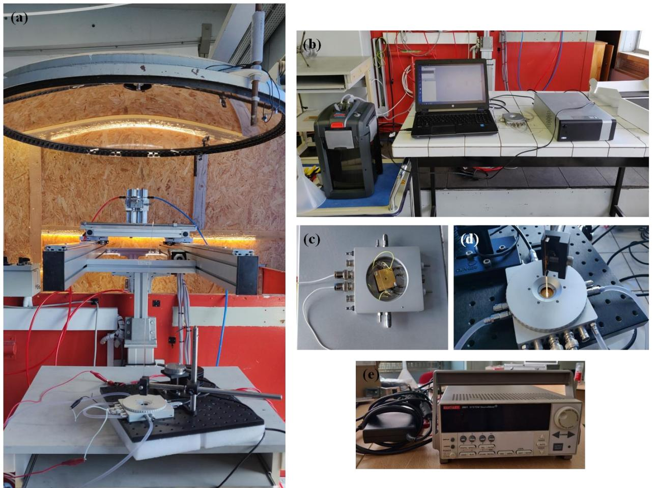
*FIGURE C-4 Experimental set-up of the high-temperature solar cells characterization (a), the temperature control system installation (b), the positioning of the solar cell on the heating plate (c), the cell illuminated by the optical fiber (d), and the Keithley 2601 (e).*
