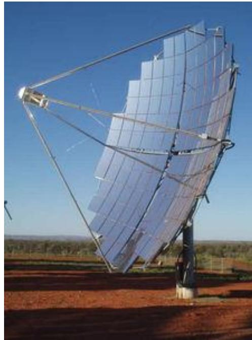
*FIGURE II-8 Parabolic mirror CPV [26].*
