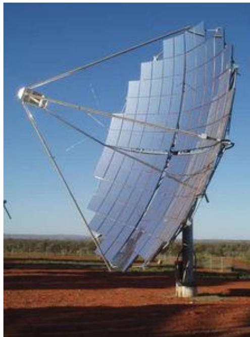
*FIGURE II-8 Parabolic mirror CPV [26].*
