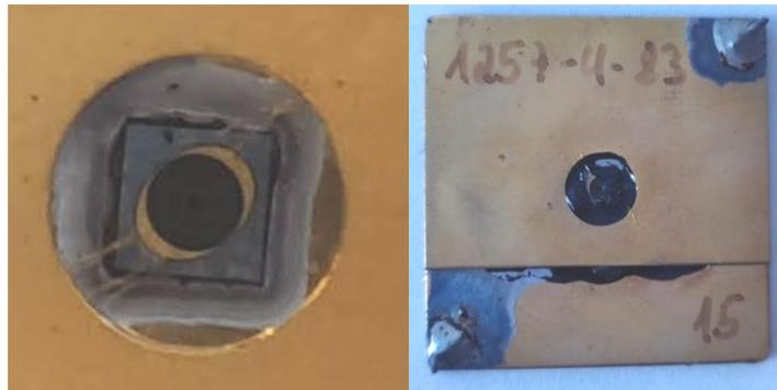
*FIGURE C-6 Solar cells at 270° (left) and at 296°C (right).*
