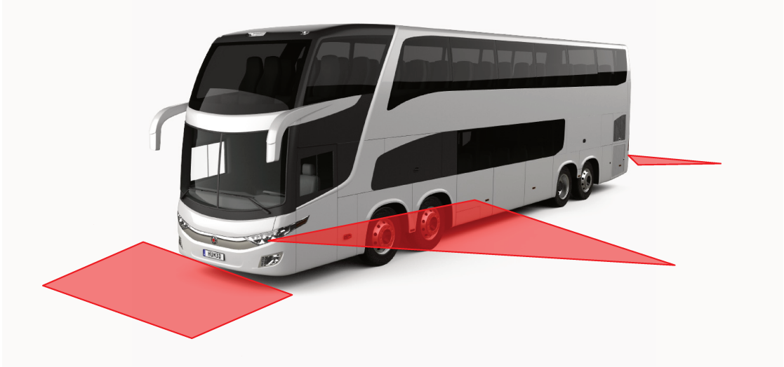
FIGURE 1.1 – A sketch showing the blind spots where the bus driver cannot visually detect road obstacles as VRUs
