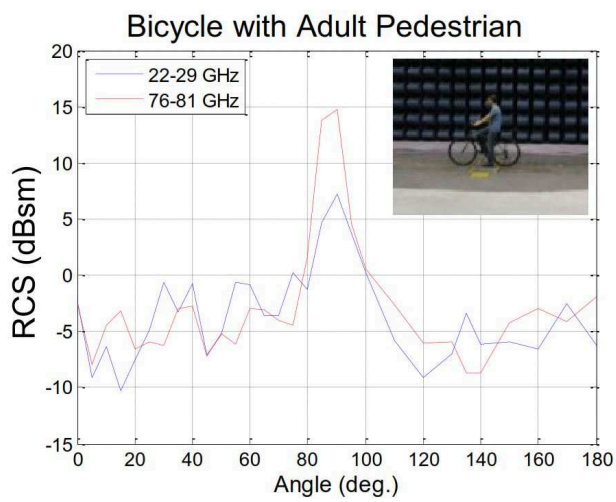
FIGURE 1.8 – Average RCS as a function of the azimuth angle of bicycle-cyclist for K-band and W-band in horizontal polarization configuration[20]
