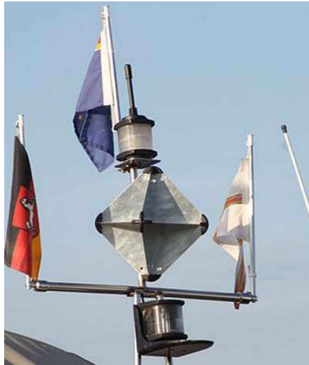
FIGURE 1.12 – A depiction of a diamond tetrahedral fixed on the mast of a yacht[23]
