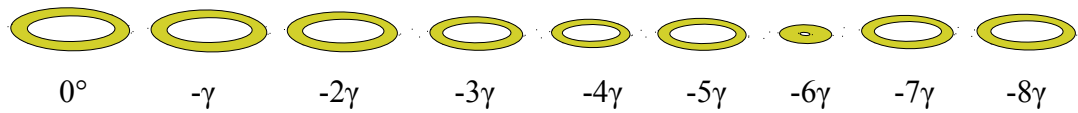
FIGURE 3.17 – Caption of the circular cells used in the design of the reflectarray
