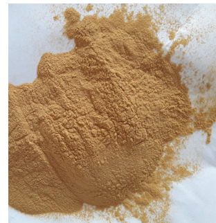
Figure. III.2 – Lignosulfonates de calcium.
