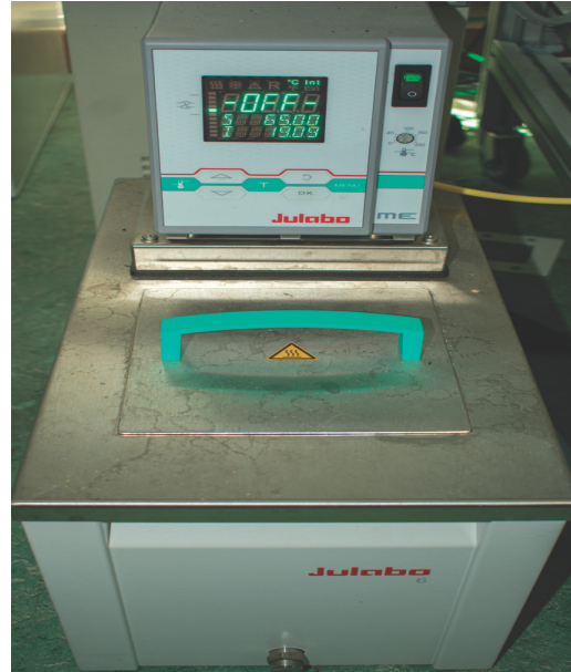
(b) Water temperature regulators
