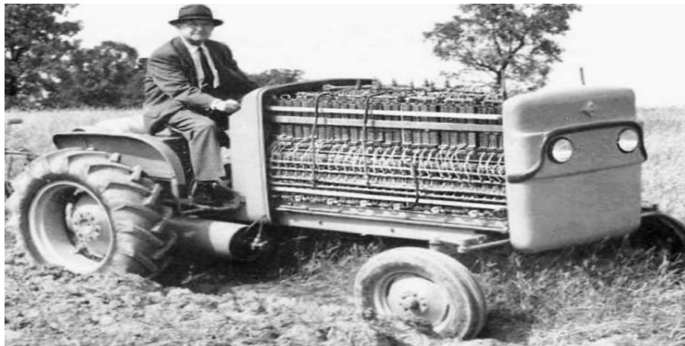
Figure 1.1: A Allis-Chalmers fuel cell powered tractor driven by Dr Harry Karl [photo produced from W. Mitchell (Ed). Fuel cells, academic press, New york, 1963]
