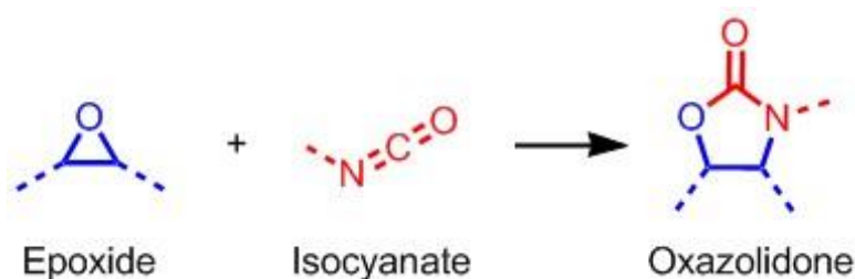
Scheme 4.1 - Oxazolidone group synthesis from epoxide and isocyanate.
