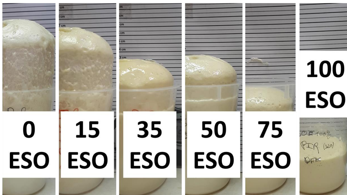
Figure S4.8 - Pictures of PUF realized with increasing content of ESO at then end of the rise. The pictures were adjusted to have an equivalent scale.
