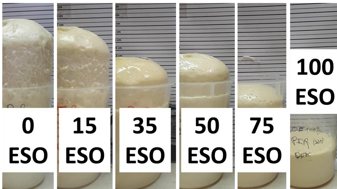
Figure S4.8 - Pictures of PUF realized with increasing content of ESO at then end of the rise. The pictures were adjusted to have an equivalent scale.
