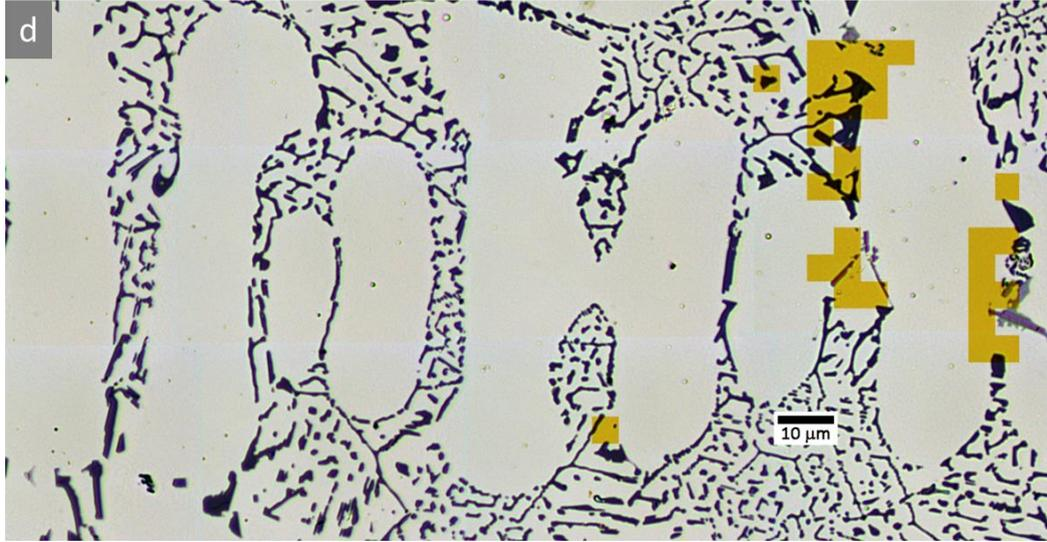
**Figure A-1.** Results of the investigation of the effect of Mg on the hardness measurements. (a) Optical micrograph of the surface after indentation. The array is constituted of 17x30 indentations. The step size is 5μm. (b) Nanohardness map (c) Young's modulus map (d) Mg map.
